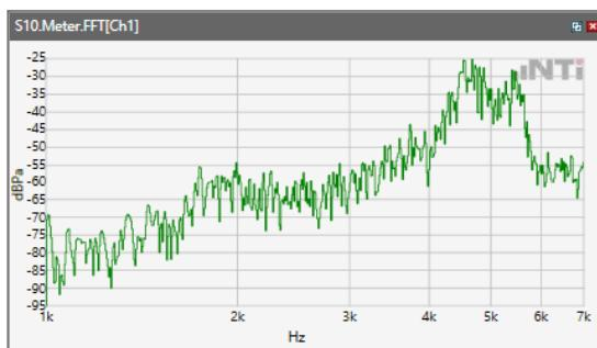
ANSI/TIA 5050-2018 \ 2N HAC ON \ WB 23.85kbps\ 5.2 Receive path – distortion and noise\ WCDM Band V
