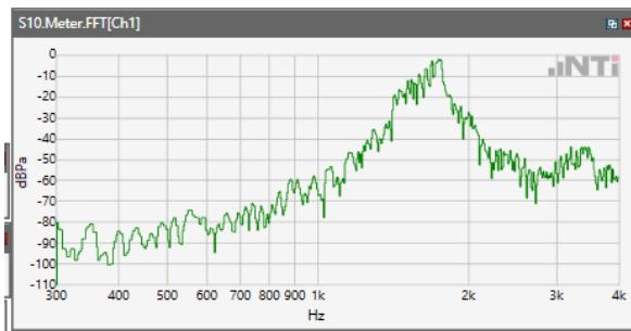
ANSI/TIA 5050-2018 \ 2N HAC ON \ WB 23.85kbps\ 5.2 Receive path – distortion and noise\ LTE Band 2
