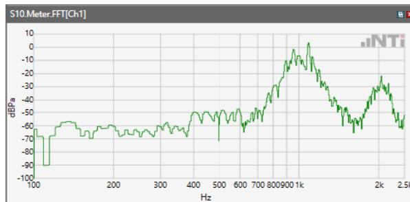
ANSI/TIA 5050-2018 \ 2N HAC ON \ WB 23.85kbps\ 5.2 Receive path – distortion and noise\GSM 1900
