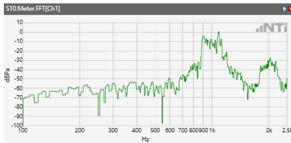
ANSI/TIA 5050-2018 \ 2N HAC ON \ WB 23.85kbps\ 5.2 Receive path – distortion and noise\ WCDM Band IV
