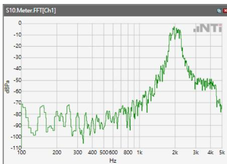
ANSI/TIA 5050-2018 \ 2N HAC ON \ WB 23.85kbps\ 5.2 Receive path – distortion and noise\ WCDM Band V
