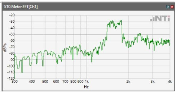
ANSI/TIA 5050-2018 \ 2N HAC ON \ WB 23.85kbps\ 5.2 Receive path – distortion and noise\LTE
