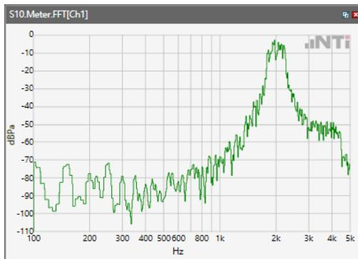
ANSI/TIA 5050-2018 \ 2N HAC ON \ WB 23.85kbps\ 5.2 Receive path – distortion and noise\LTE Band 71
