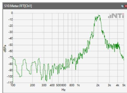
ANSI/TIA 5050-2018 \ 2N HAC ON \ WB 23.85kbps\ 5.2 Receive path – distortion and noise\ LTE Band 2
