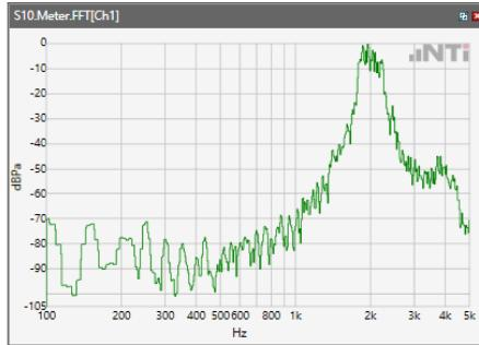
ANSI/TIA 5050-2018 \ 2N HAC ON \ WB 23.85kbps\ 5.2 Receive path – distortion and noise\WCDM Band II
