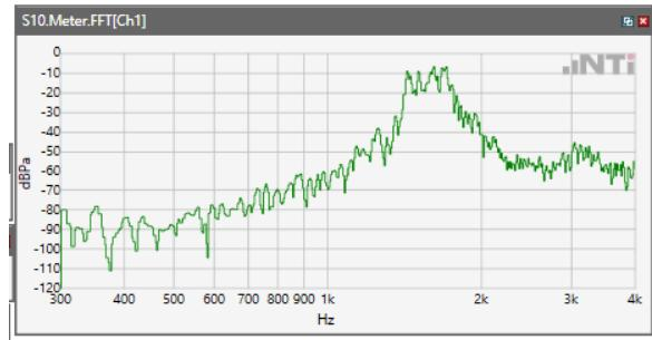
ANSI/TIA 5050-2018 \ 2N HAC ON \ WB 23.85kbps\ 5.2 Receive path – distortion and noise\GSM 1900
