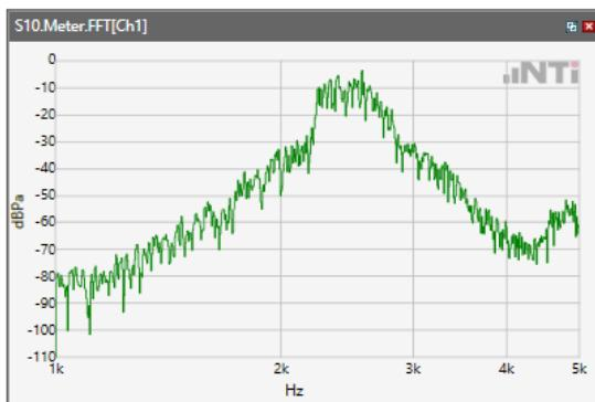
ANSI/TIA 5050-2018 \ 2N HAC ON \ NB 12.2kbps\ 5.2 Receive path – distortion and noise\LTE Band 7..
