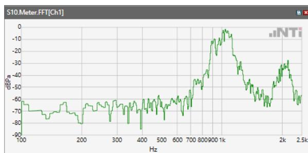
ANSI/TIA 5050-2018 \ 2N HAC ON \ WB 23.85kbps\ 5.2 Receive path – distortion and noise\ LTE Band 2
