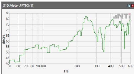
ANSI/TIA 5050-2018 \ 2N HAC ON \ NB 12.2kbps\ 5.2 Receive path – distortion and noise\LTE Band 7.
