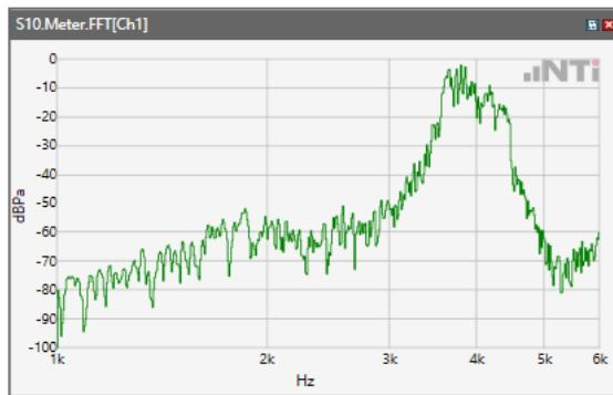
ANSI/TIA 5050-2018 \ 2N HAC ON \ WB 23.85kbps\ 5.2 Receive path – distortion and noise\LTE
