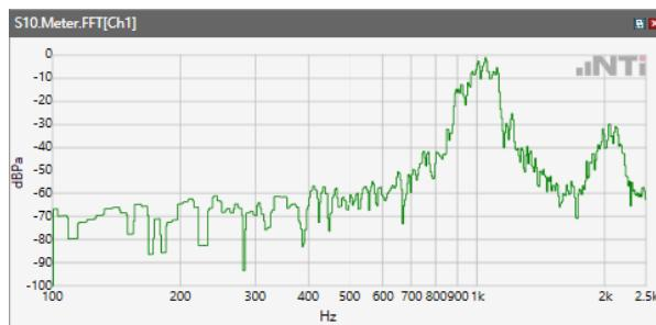
ANSI/TIA 5050-2018 \ 2N HAC ON \ WB 23.85kbps\ 5.2 Receive path – distortion and noise\LTE Band 71
