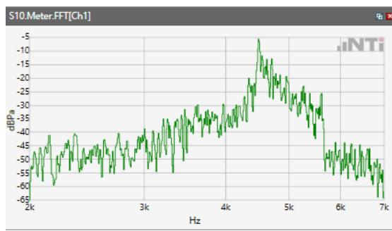
ANSI/TIA 5050-2018 \ 8N HAC OFF \ WB 23.85 kbps\ 5.2 Receive path – distortion and noise\WCDMA Band II
