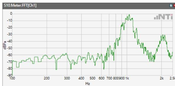
ANSI/TIA 5050-2018 \ 2N HAC ON \ WB 23.85kbps\ 5.2 Receive path – distortion and noise\WCDM Band II
