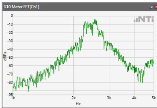
ANSI/TIA 5050-2018 \ 2N HAC ON \ WB 23.85kbps\ 5.2 Receive path – distortion and noise\ LTE Band 66
