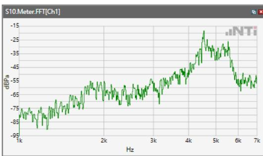
ANSI/TIA 5050-2018 \ 2N HAC ON \ WB 23.85kbps\ 5.2 Receive path – distortion and noise\ LTE Band 2
