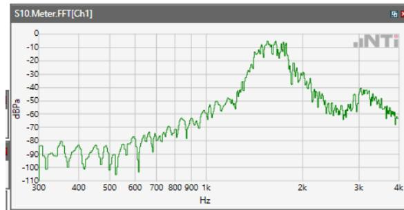
ANSI/TIA 5050-2018 \ 2N HAC ON \ WB 23.85kbps\ 5.2 Receive path – distortion and noise\WCDM Band II
