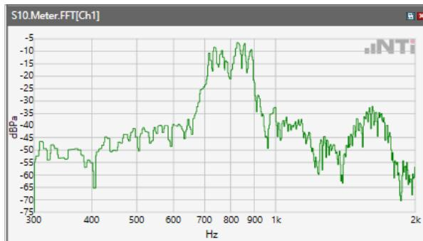
ANSI/TIA 5050-2018 \ 2N HAC ON \ WB 23.85kbps\ 5.2 Receive path – distortion and noise\LTE Band 71
