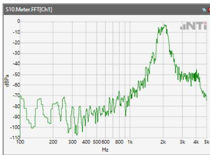
ANSI/TIA 5050-2018 \ 2N HAC ON \ WB 23.85kbps\ 5.2 Receive path – distortion and noise\WLAN 2.4GHz
