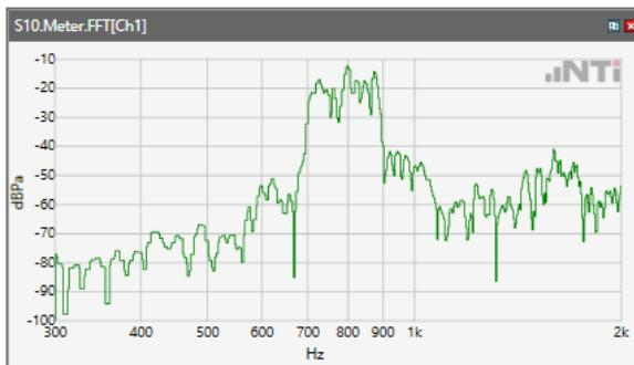
ANSI/TIA 5050-2018 \ 2N HAC ON \ WB 23.85kbps\ 5.2 Receive path – distortion and noise\LTE Band 7
