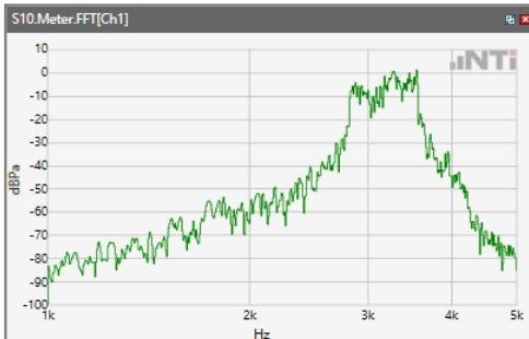
ANSI/TIA 5050-2018 \ 2N HAC ON \ WB 23.85kbps\ 5.2 Receive path – distortion and noise\WCDM Band II
