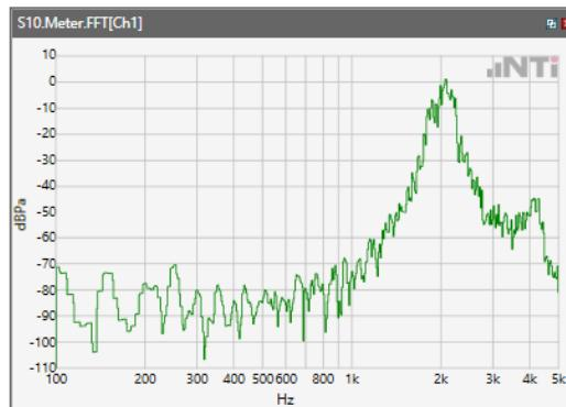
ANSI/TIA 5050-2018 \ 2N HAC ON \ NB 12.2kbps\ 5.2 Receive path – distortion and noise\LTE Band 66
