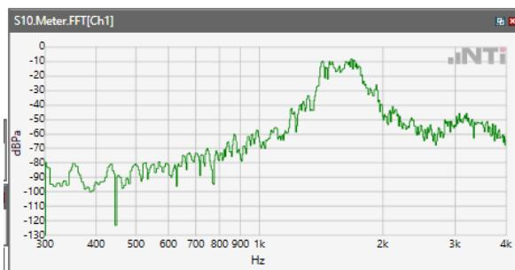
ANSI/TIA 5050-2018 \ 2N HAC ON \ WB 23.85kbps\ 5.2 Receive path – distortion and noise\ WCDM Band V
