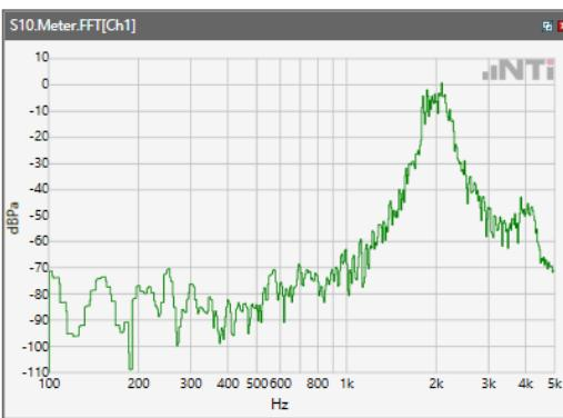
ANSI/TIA 5050-2018 \ 2N HAC ON \ NB 12.2kbps\ 5.2 Receive path – distortion and noise\WCDMA Band II
