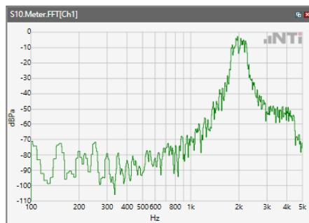
ANSI/TIA 5050-2018 \ 2N HAC ON \ WB 23.85kbps\ 5.2 Receive path – distortion and noise\LTE Band 71
