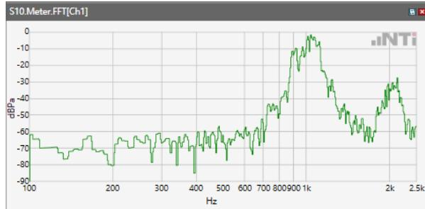
ANSI/TIA 5050-2018 \ 2N HAC ON \ WB 23.85kbps\ 5.2 Receive path – distortion and noise\ LTE Band 66
