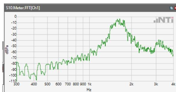
ANSI/TIA 5050-2018 \ 2N HAC ON \ WB 23.85kbps\ 5.2 Receive path – distortion and noise\ WCDM Band IV
