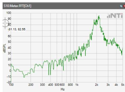
ANSI/TIA 5050-2018 \ 8N HAC OFF \ WB 23.85 kbps\ 5.2 Receive path – distortion and noise\LTE Band 2
