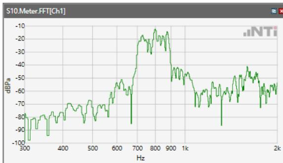
ANSI/TIA 5050-2018 \ 2N HAC ON \ WB 23.85kbps\ 5.2 Receive path – distortion and noise\LTE Band 5
