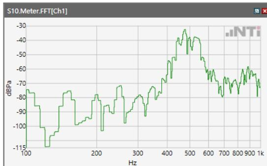
ANSI/TIA 5050-2018 \ 2N HAC ON \ WB 23.85kbps\ 5.2 Receive path – distortion and noise\LTE
