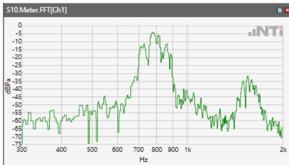
ANSI/TIA 5050-2018 \ 2N HAC ON \ WB 23.85kbps\ 5.2 Receive path – distortion and noise\ LTE Band 66
