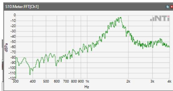
ANSI/TIA 5050-2018 \ 2N HAC ON \ NB 12.2kbps\ 5.2 Receive path – distortion and noise\LTE Band 7.
