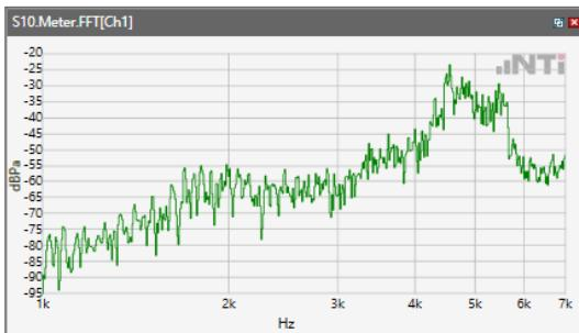
ANSI/TIA 5050-2018 \ 2N HAC ON \ WB 23.85kbps\ 5.2 Receive path – distortion and noise\GSM 1900
