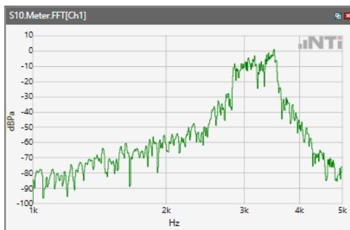
ANSI/TIA 5050-2018 \ 2N HAC ON \ WB 23.85kbps\ 5.2 Receive path – distortion and noise\ WCDM Band V
