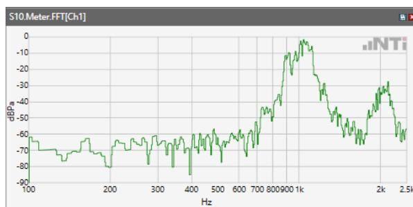
ANSI/TIA 5050-2018 \ 2N HAC ON \ WB 23.85kbps\ 5.2 Receive path – distortion and noise\WLAN 2.4GHz
