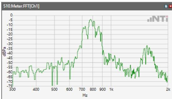
ANSI/TIA 5050-2018 \ 2N HAC ON \ WB 23.85kbps\ 5.2 Receive path – distortion and noise\ LTE Band 2
