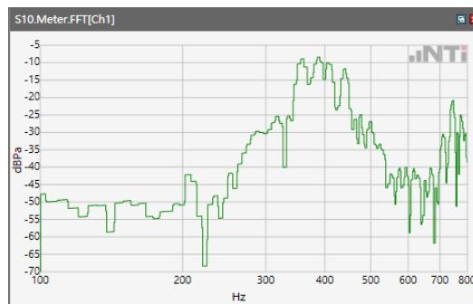
ANSI/TIA 5050-2018 \ 2N HAC ON \ WB 23.85kbps\ 5.2 Receive path – distortion and noise\ WCDM Band V
