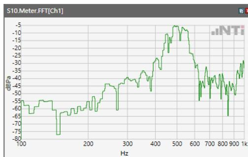
ANSI/TIA 5050-2018 \ 2N HAC ON \ WB 23.85kbps\ 5.2 Receive path – distortion and noise\ WCDM Band IV
