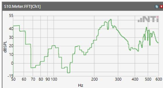
ANSI/TIA 5050-2018 \ 2N HAC ON \ WB 23.85kbps\ 5.2 Receive path – distortion and noise\WCDM Band II
