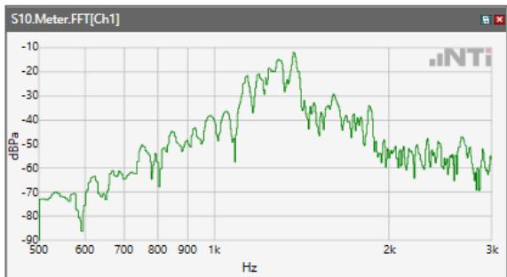
ANSI/TIA 5050-2018 \ 2N HAC ON \ WB 23.85kbps\ 5.2 Receive path – distortion and noise\ WCDM Band V
