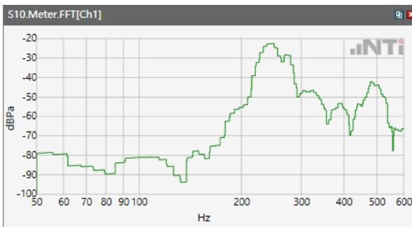
ANSI/TIA 5050-2018 \ 2N HAC ON \ WB 23.85kbps\ 5.2 Receive path – distortion and noise\LTE
