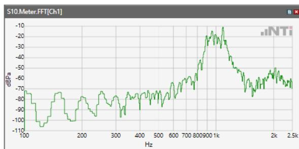
ANSI/TIA 5050-2018 \ 2N HAC ON \ WB 23.85kbps\ 5.2 Receive path – distortion and noise\LTE Band 12
