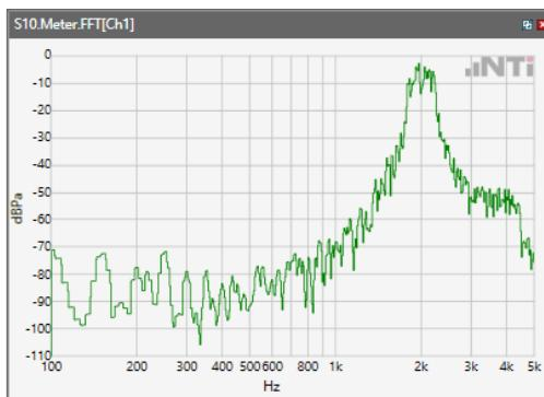
ANSI/TIA 5050-2018 \ 2N HAC ON \ WB 23.85kbps\ 5.2 Receive path – distortion and noise\LTE
