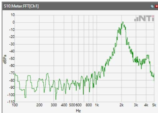
ANSI/TIA 5050-2018 \ 2N HAC ON \ NB 12.2kbps\ 5.2 Receive path – distortion and noise\GSM 1900
