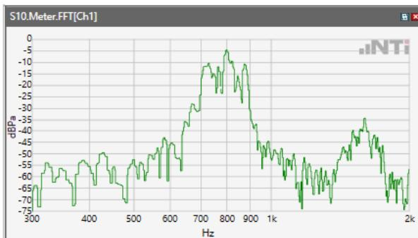
ANSI/TIA 5050-2018 \ 2N HAC ON \ NB 12.2kbps\ 5.2 Receive path – distortion and noise\LTE Band 7
