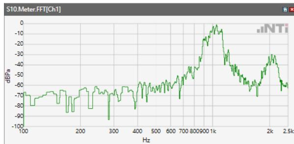
ANSI/TIA 5050-2018 \ 2N HAC ON \ WB 23.85kbps\ 5.2 Receive path – distortion and noise\LTE Band 7
