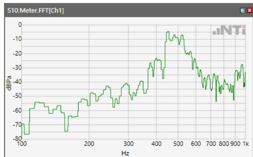
ANSI/TIA 5050-2018 \ 2N HAC ON \ WB 23.85kbps\ 5.2 Receive path – distortion and noise\WCDM Band II
