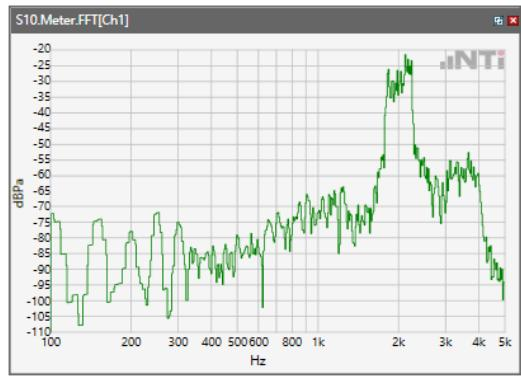
ANSI/TIA 5050-2018 \ 2N HAC ON \ NB 12.2kbps\ 5.2 Receive path – distortion and noise\LTE Band 5
