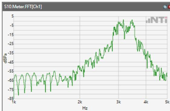
ANSI/TIA 5050-2018 \ 8N HAC OFF \ WB 23.85 kbps\ 5.2 Receive path – distortion and noise\WLAN
