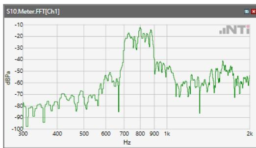
ANSI/TIA 5050-2018 \ 2N HAC ON \ WB 23.85kbps\ 5.2 Receive path – distortion and noise\ WCDM Band IV
