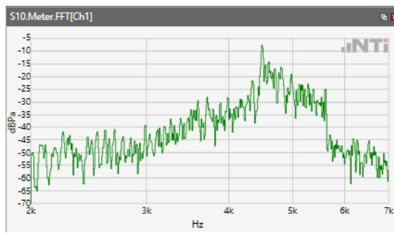
ANSI/TIA 5050-2018 \ 8N HAC OFF \ WB 23.85 kbps\ 5.2 Receive path – distortion and noise\WCDMA Band IV
