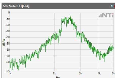
ANSI/TIA 5050-2018 \ 2N HAC ON \ WB 23.85kbps\ 5.2 Receive path – distortion and noise\ WCDM Band IV
