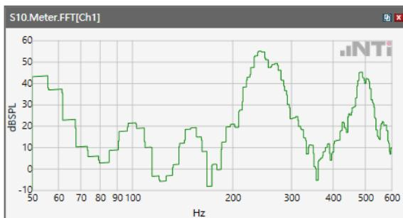
ANSI/TIA 5050-2018 \ 2N HAC ON \ WB 23.85kbps\ 5.2 Receive path – distortion and noise\ WCDM Band IV
