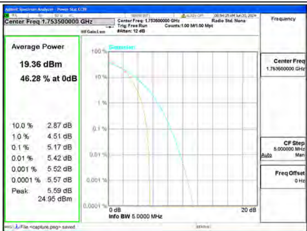
B4 / 3MHz / High CH / 16QAM
