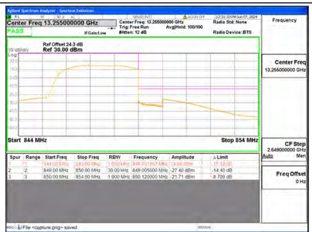
B5 / 3MHz / High CH / QPSK / FULL RB
