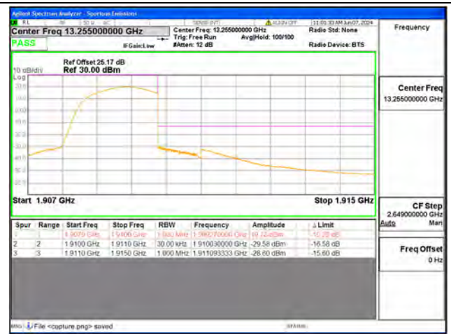
B2 / 1.4MHz / High CH / QPSK / FULL RB
