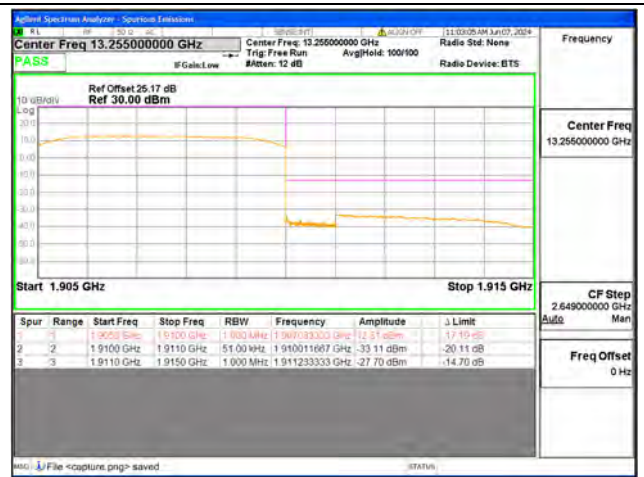
B2 / 5MHz / High CH / QPSK / FULL RB
