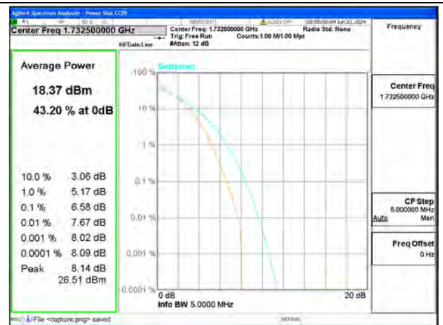
B4 / 5MHz / Mid CH / 64QAM
