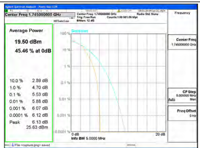
B66 / 3MHz / Mid CH / 16QAM
