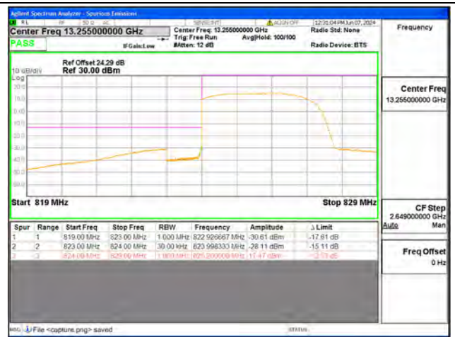
B5 / 3MHz / Low CH / QPSK / FULL RB
