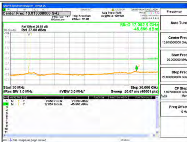
B7-30M-20G / 20MHz / High CH / QPSK
