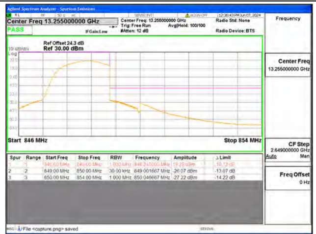
B5 / 1.4MHz / High CH / QPSK / FULL RB
