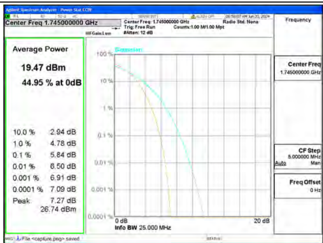
B4 / 20MHz / High CH / 16QAM
