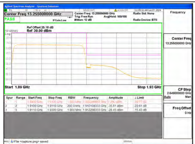
B2 / 20MHz / High CH / QPSK / FULL RB
