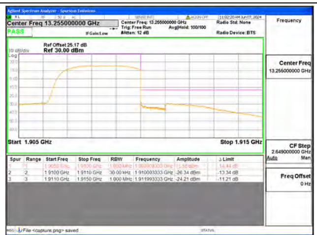
B2 / 3MHz / High CH / QPSK / FULL RB
