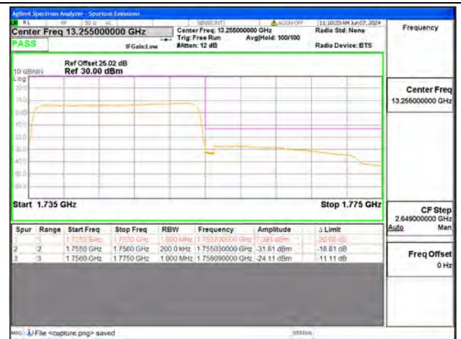
B4 / 20MHz / High CH / QPSK / FULL RB
