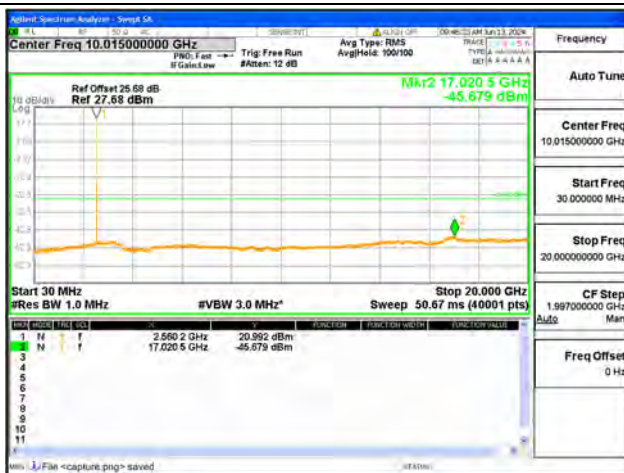
B7-30M-20G / 10MHz / High CH / QPSK
