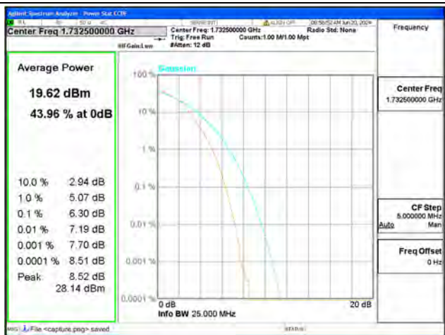
B4 / 15MHz / Mid CH / 16QAM
