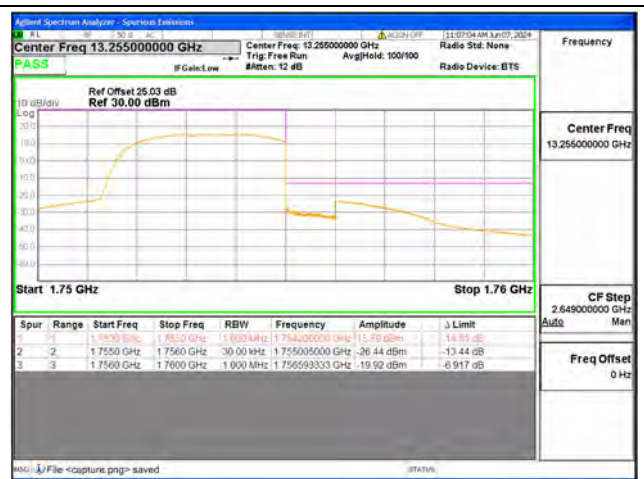
B4 / 3MHz / High CH / QPSK / FULL RB
