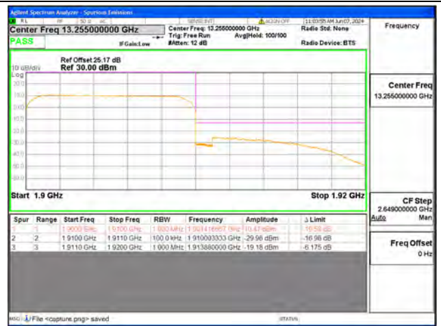
B2 / 10MHz / High CH / QPSK / FULL RB
