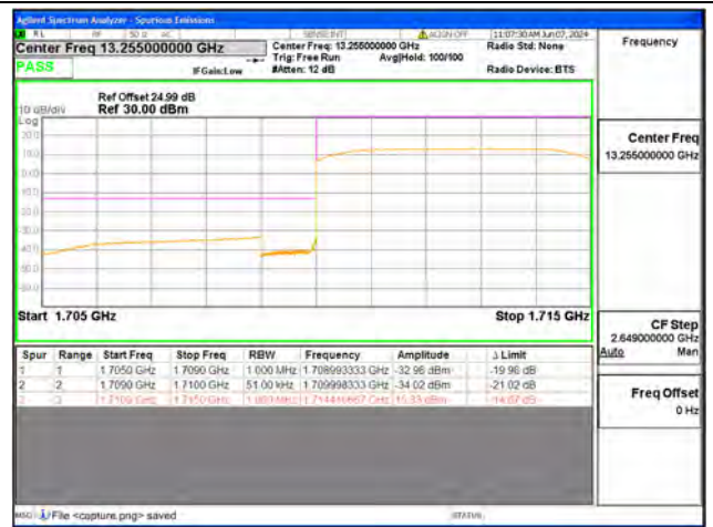
B4 / 5MHz / Low CH / QPSK / FULL RB
