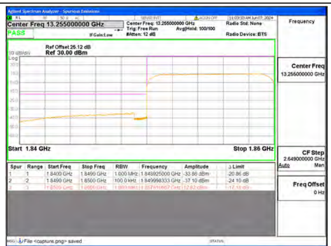
B2 / 10MHz / Low CH / QPSK / FULL RB
