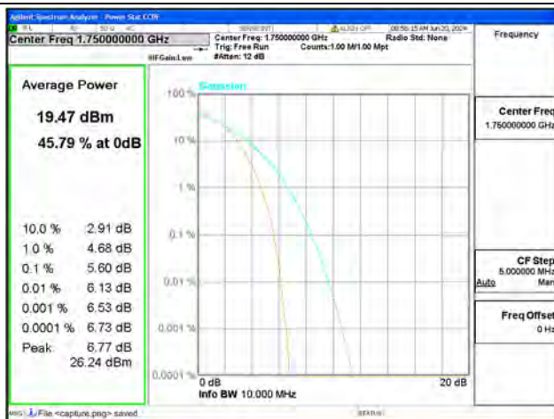
B4 / 10MHz / High CH / 16QAM
