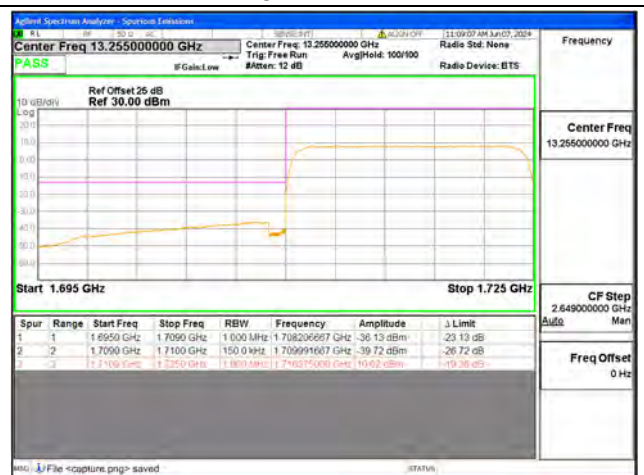
B4 / 15MHz / Low CH / QPSK / FULL RB
