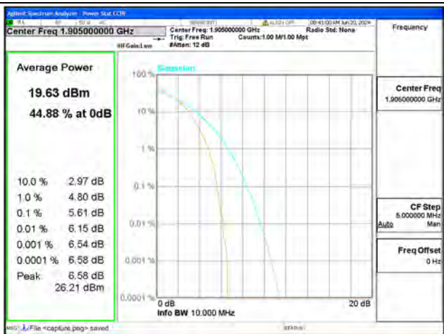
B2 / 10MHz / High CH / 16QAM
