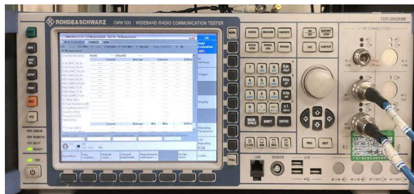
CMW 500 (2G/3G/4G Test Equipment)
