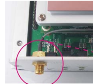
RF cable mounted at the front panel
