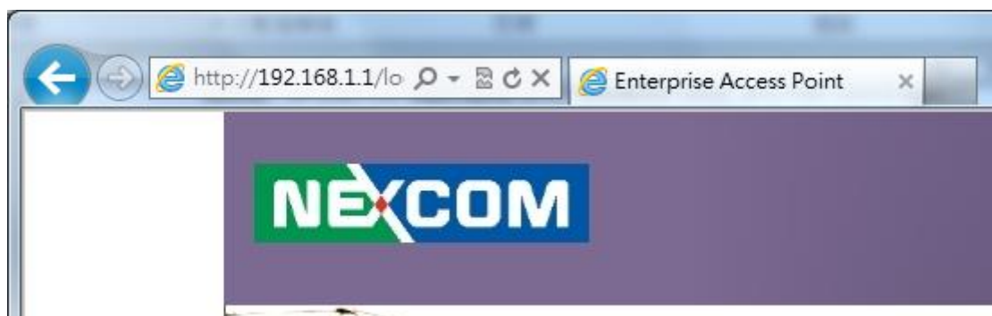
Example of entering the AP's default IP Address into a web browser
