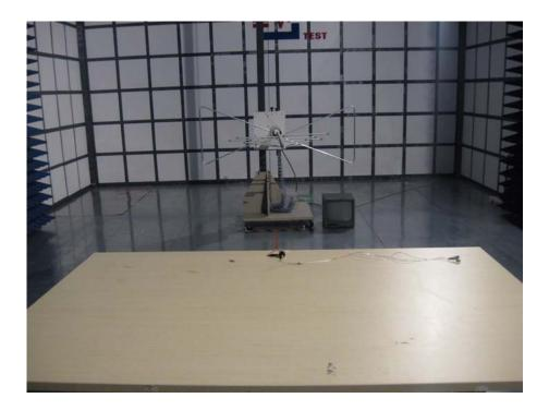
Radiation Emission Test Setup (Above 1GHz)
