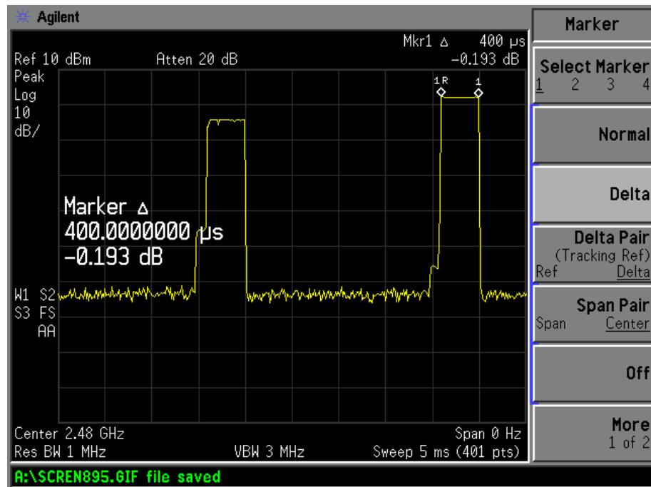
$$\text{DH1 time slot} = 0.40 \text{ (ms)} * (1600/(79)) * 31.6 = 256 \text{ (ms)} < 400 \text{ (ms)}$$
