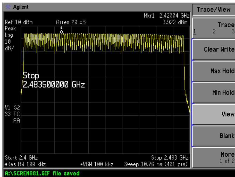
Channel Spacing (Low CH=1MHz)
