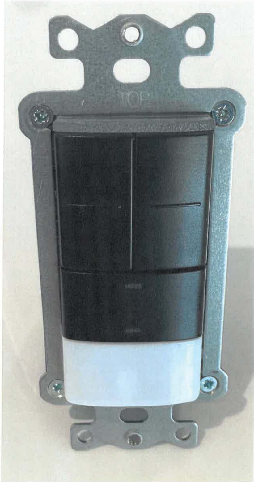
Metal bracket identical for all variants. Front plastic in this picture, for reference, is NXSMIR-LH2-BK
