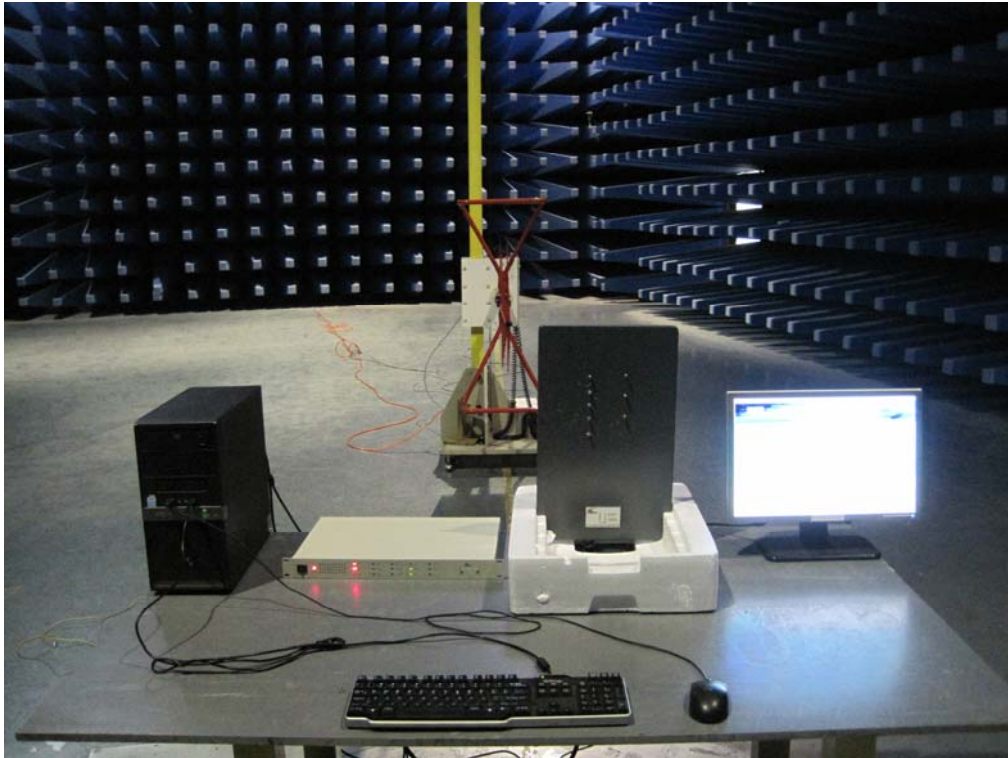
Radiated Spurious Emissions Test Setup (30MHz-1GHz)
