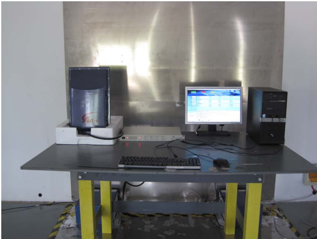
Conducted Emissions Test Setup Front View
