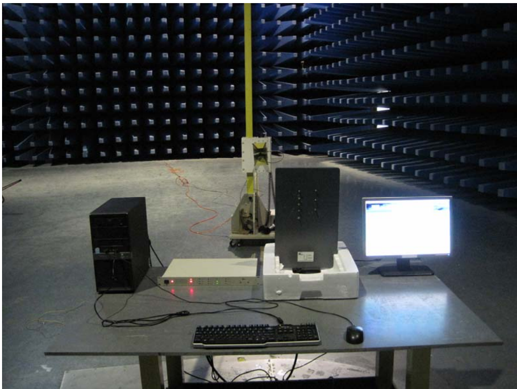
Radiated Spurious Emissions Test Setup (Above 1GHz)
