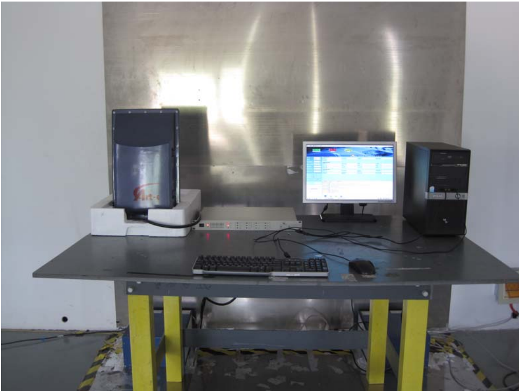
Conducted Emissions Test Setup Front View
