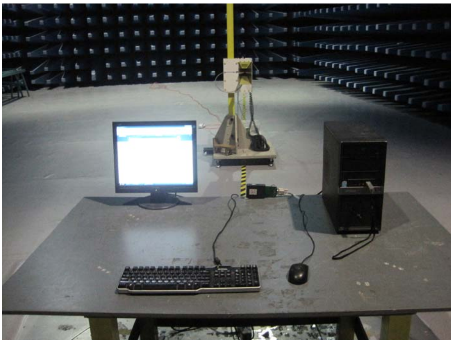
Radiated Spurious Emissions Test Setup (30MHz-1GHz)
