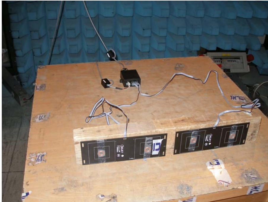
Photo 3. RE test setup in Anechoic chamber.
