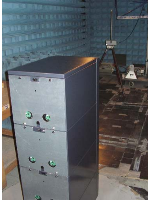
Photo 1. RE test setup.
