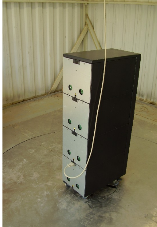
Photo 3. RE test setup on OATS.
