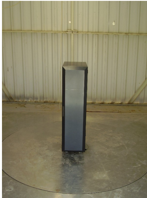
Photo 2. RE test setup on OATS.
