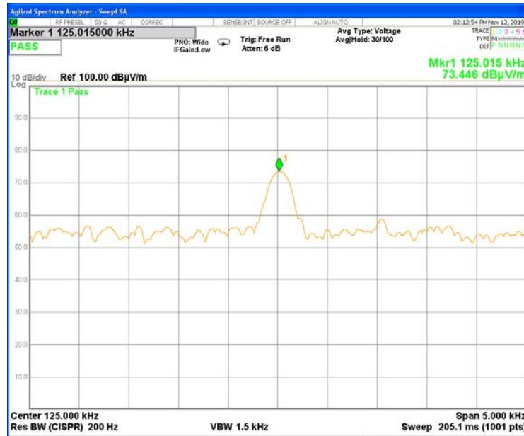
Plot # 1. Field strength of fundamental frequency 125 kHz.
