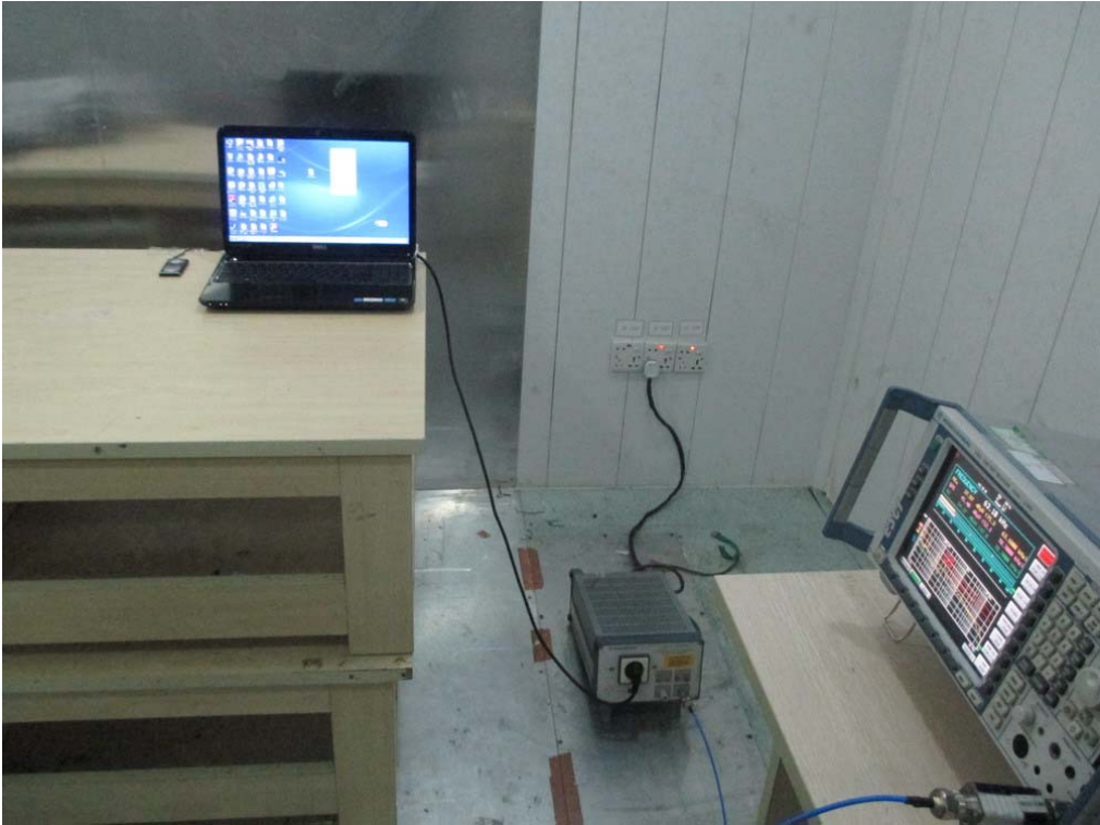
FCC RADIATED EMISSION TEST SETUP
