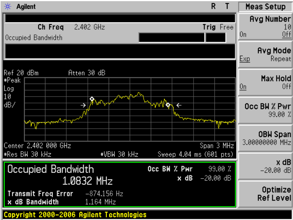
TEST PLOT OF BANDWIDTH FOR LOW CHANNEL
