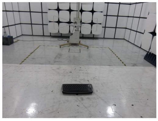
RADIATED EMISSION TEST SETUP ABOVE 1GHz
