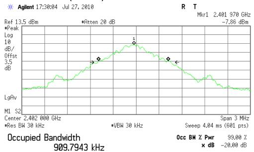
Transmit Freq Error -33.862 kHz x dB Bandwidth 959.288 kHz
