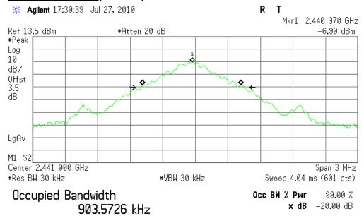
Transmit Freq Error -32.318 kHz x dB Bandwidth 950.672 kHz
