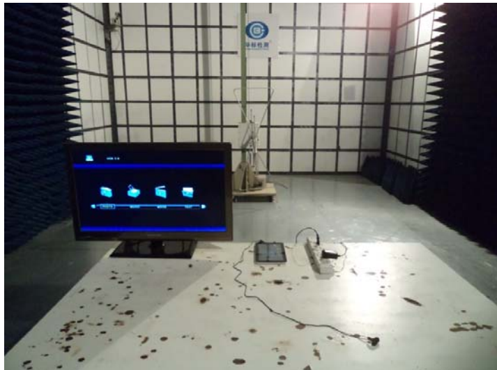
Radiated Emission 30MHz To 1G
