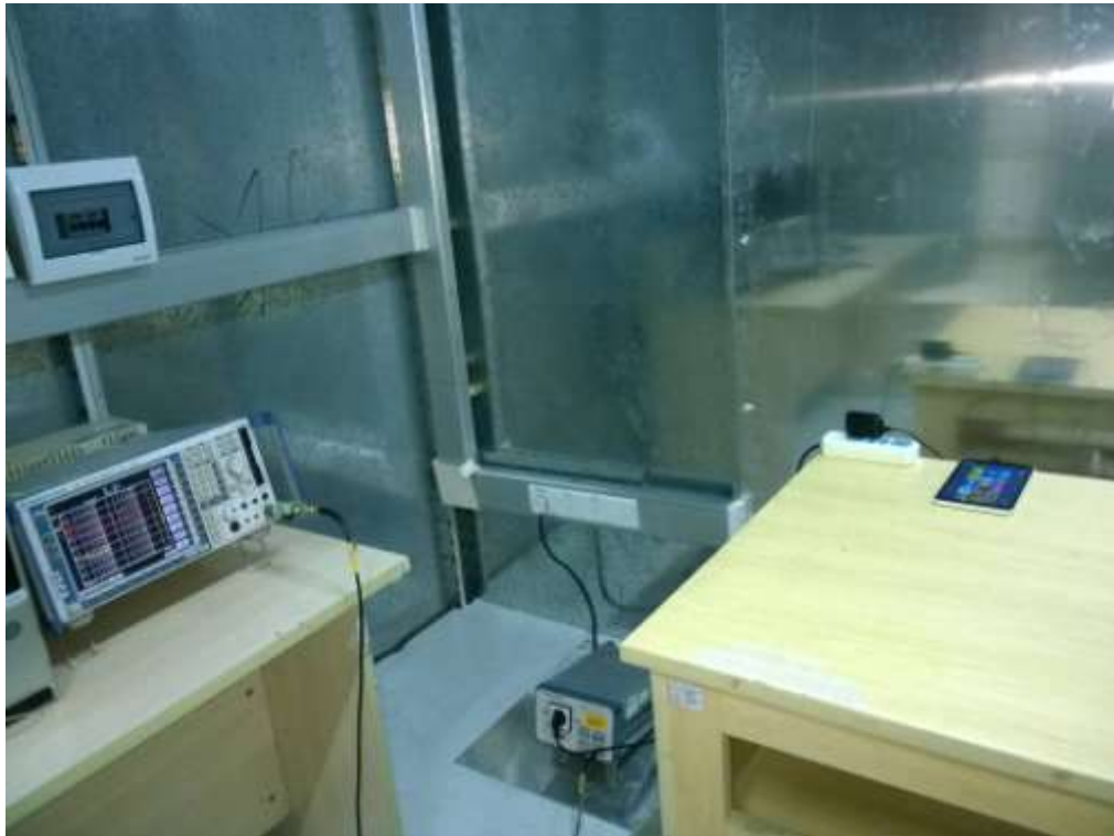
FCC RADIATED EMISSION TEST SETUP
