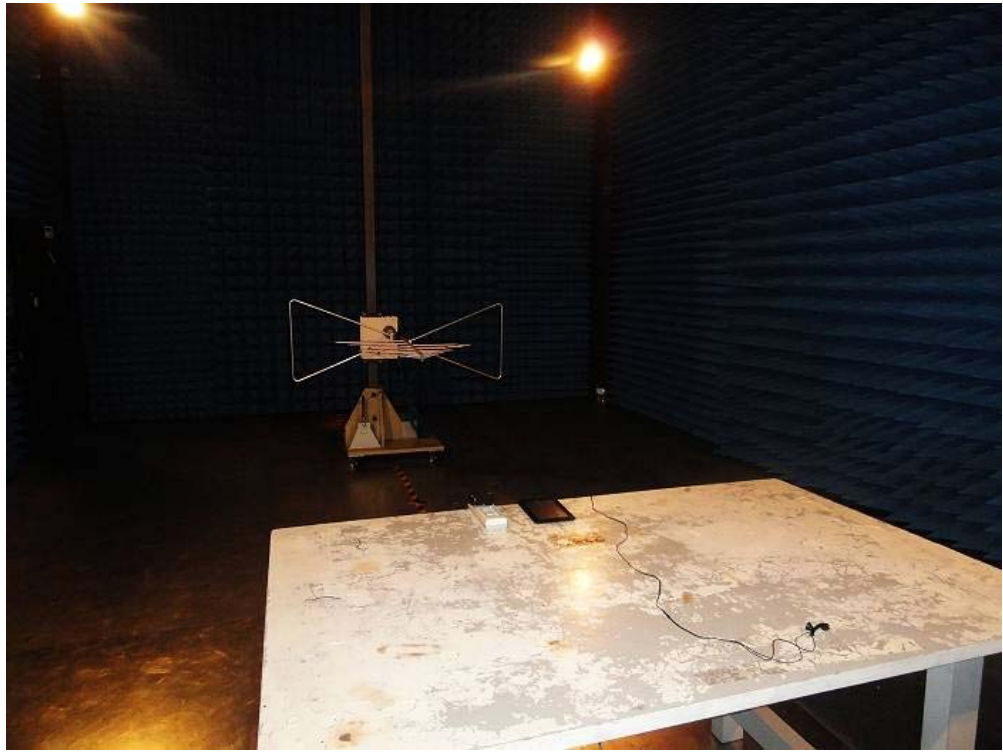
Radiated Emission Test Setup:
