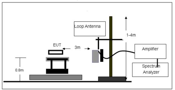
(B) Radiated Emission Test-Up Frequency 30MHz~1GHz
