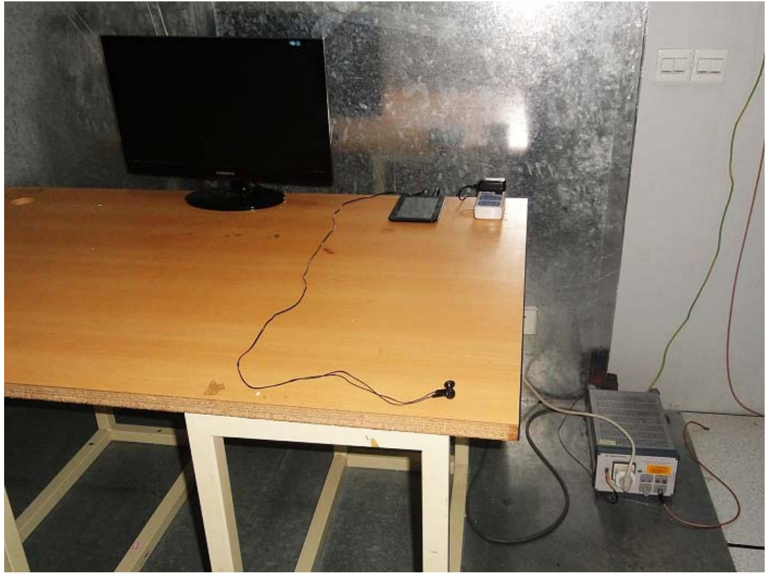
Conducted Emission Test Setup:
