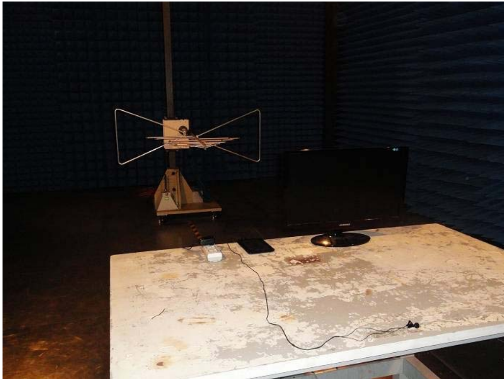
Radiated Emission Test Setup:
