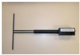
Figure 1 – Satimo COMOSAR Validation Dipole
