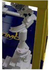
*Note:* A simulating human hand is not used due to the complex anatomical and geometrical structure of the hand that may produced infinite number of configurations [10]. To produce the worst-case condition (the hand absorbs antenna output power), the hand is omitted during the tests.
