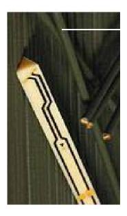
Construction Symmetrical design with triangular Core. Built-in shielding against static charges Calibration in air from 100 MHz to 2.5 GHz. In brain and muscle simulating tissue at frequencies from 800 to 6000 MHz (accuracy of 8%).
