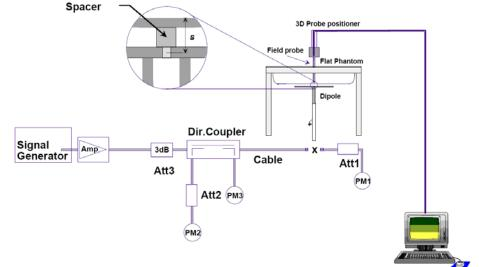
Fig 8.1 System Setup for System Evaluation
