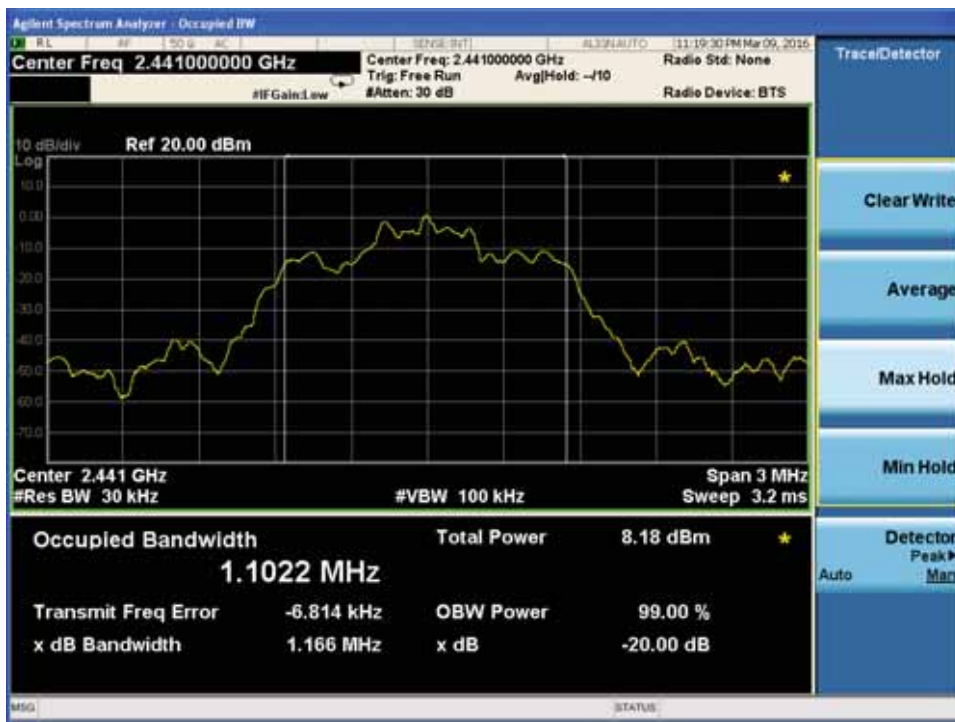
20dB Bandwidth plot on channel 39
