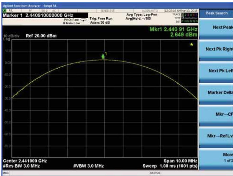
Peak output Power plot on channel 39
