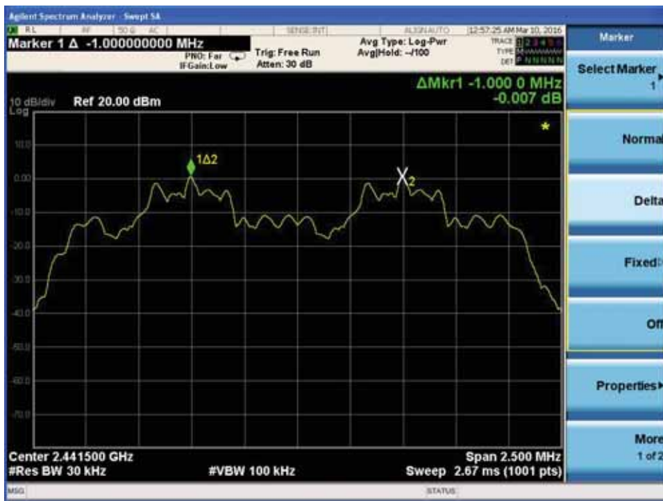
Channel Separation plot on channel 39-40
