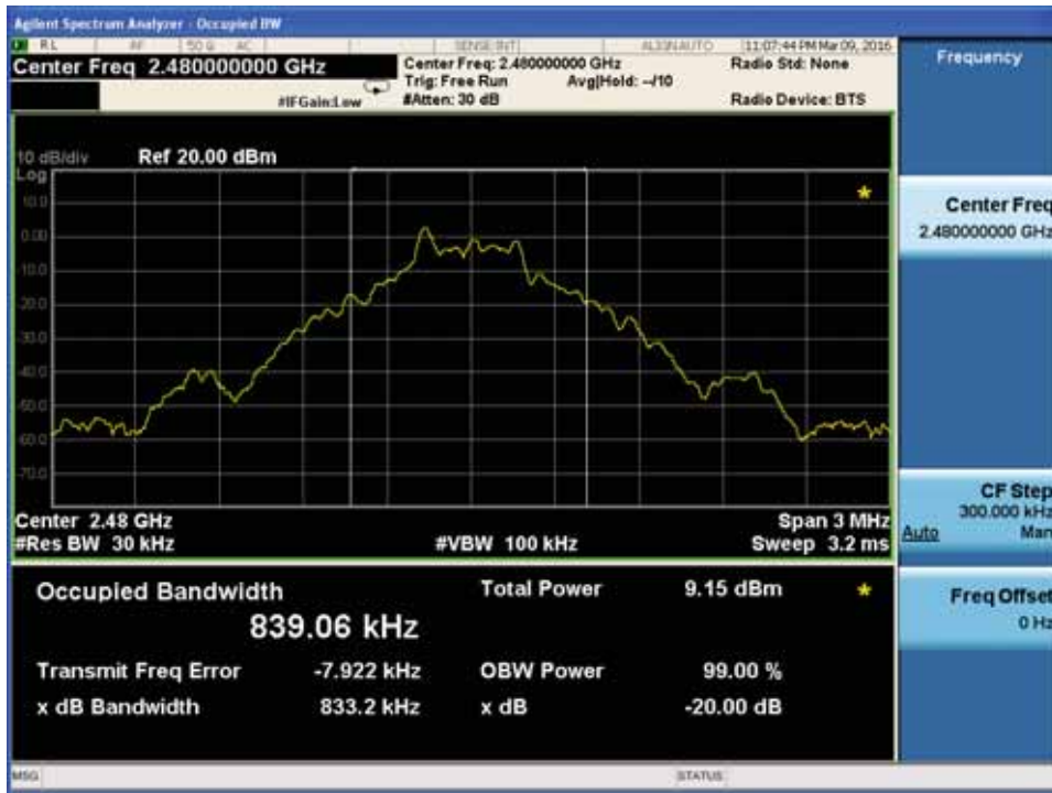
20dB Bandwidth plot on channel 00
