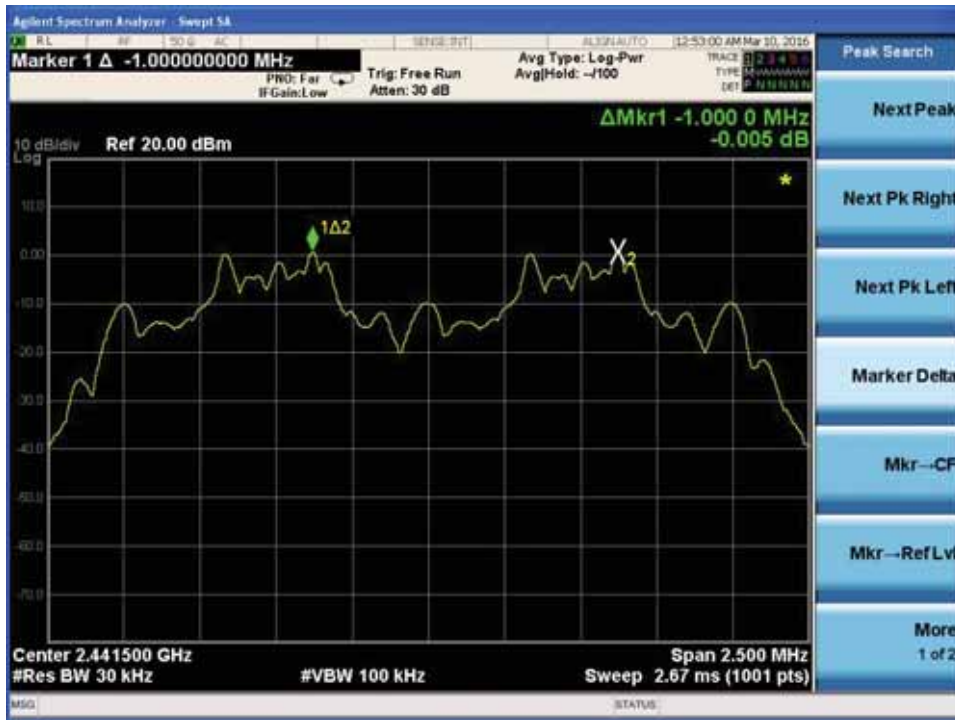
Channel Separation plot on channel 77-78
