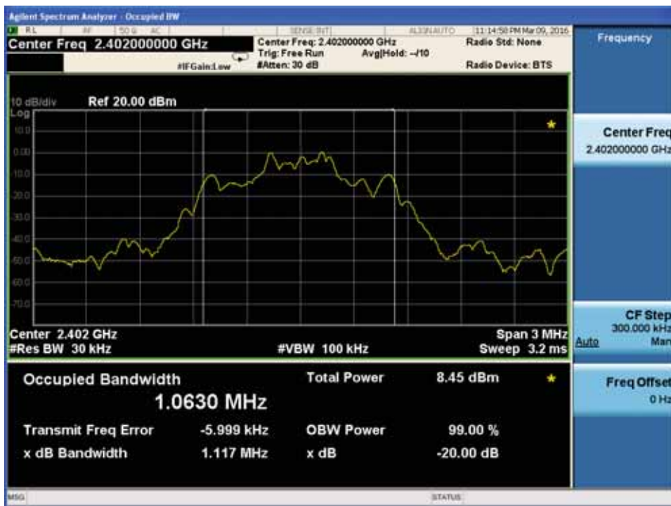
20dB Bandwidth plot on channel 00
