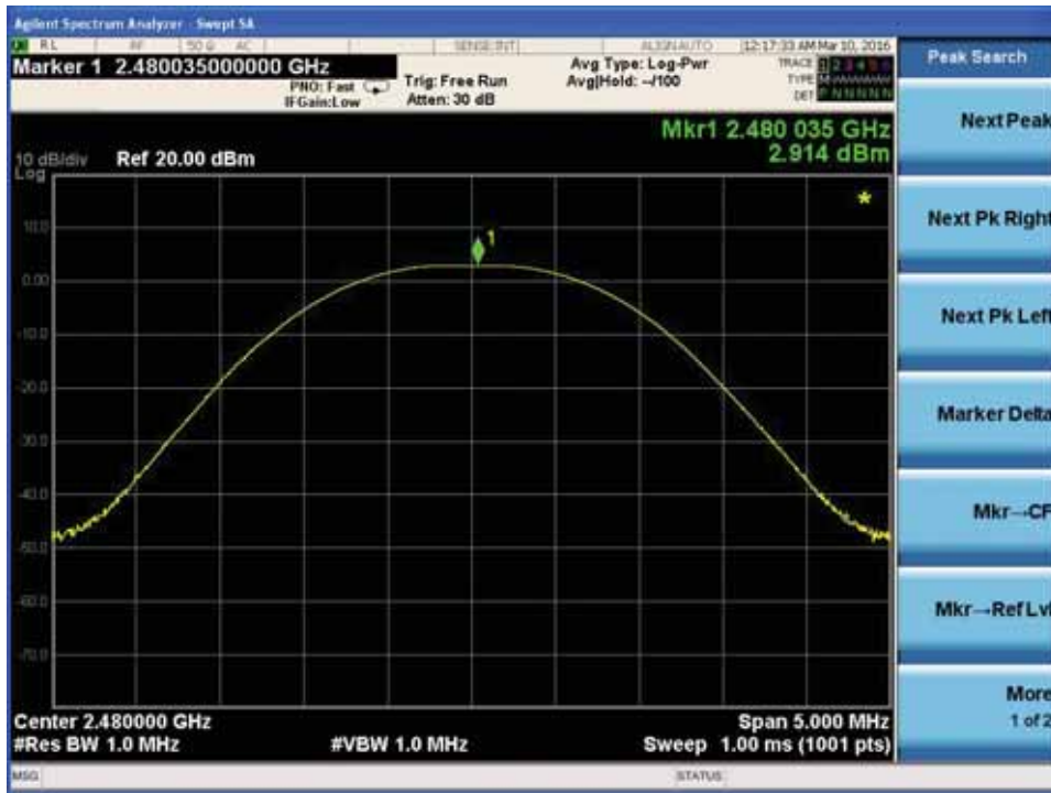
Peak output Power plot on channel 00
