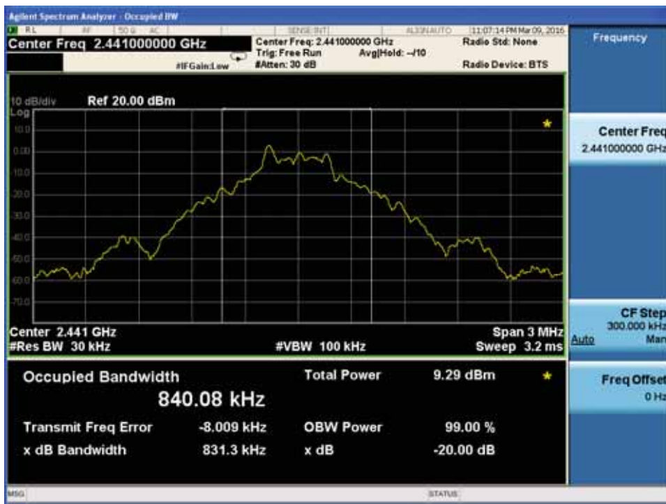
20dB Bandwidth plot on channel 39
