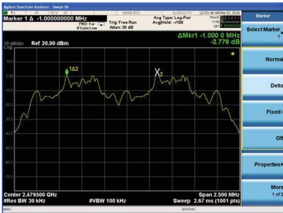
Channel Separation plot on channel 77-78
