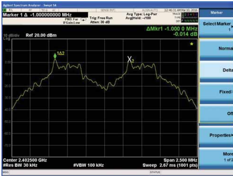
Channel Separation plot on channel 39-40
