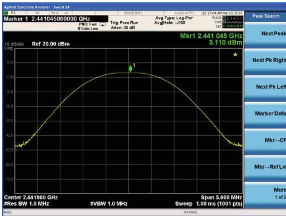
Peak output Power plot on channel 39
