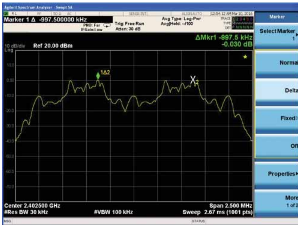
Channel Separation plot on channel 00-01
