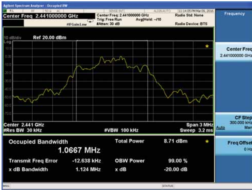
20dB Bandwidth plot on channel 78
