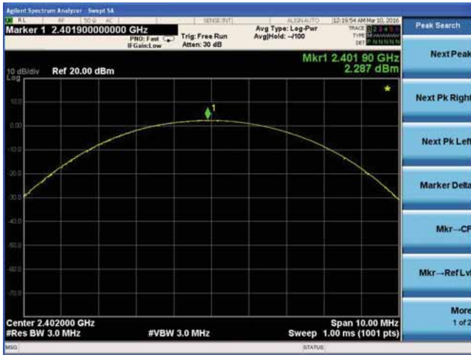
Peak output Power plot on channel 39
