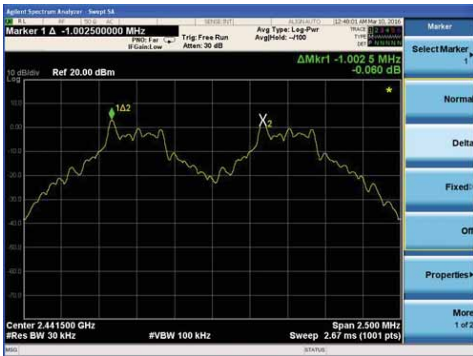
Channel Separation plot on channel 39-40
