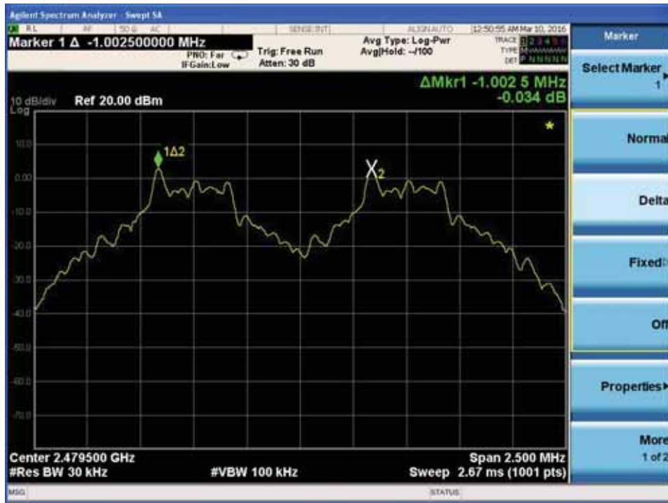
Channel Separation plot on channel 00-01
