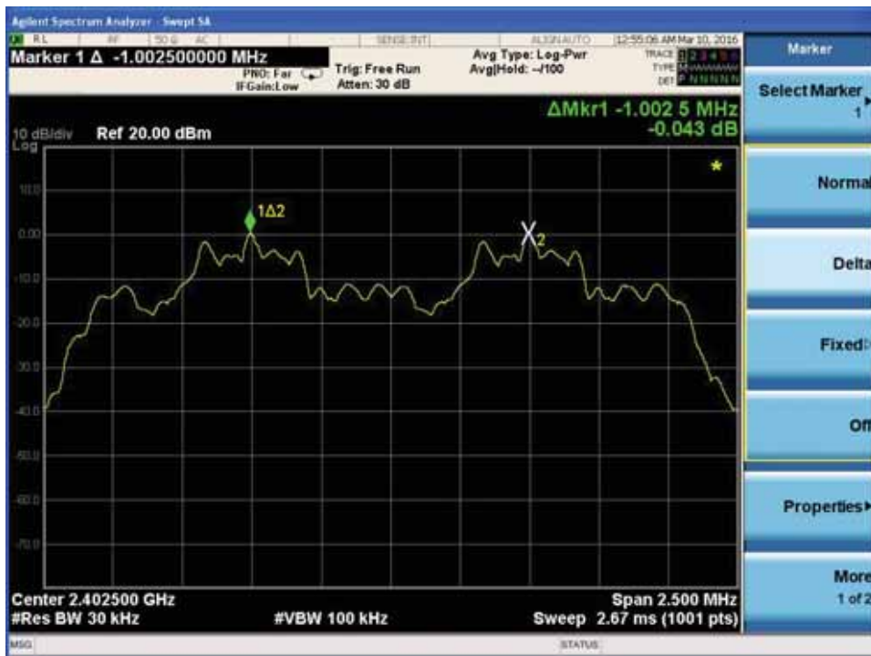
Channel Separation plot on channel 39-40
