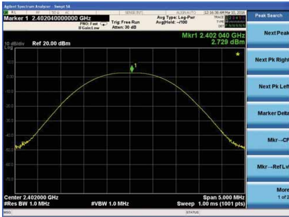
Peak output Power plot on channel 39
