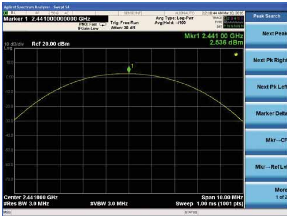
Peak output Power plot on channel 78
