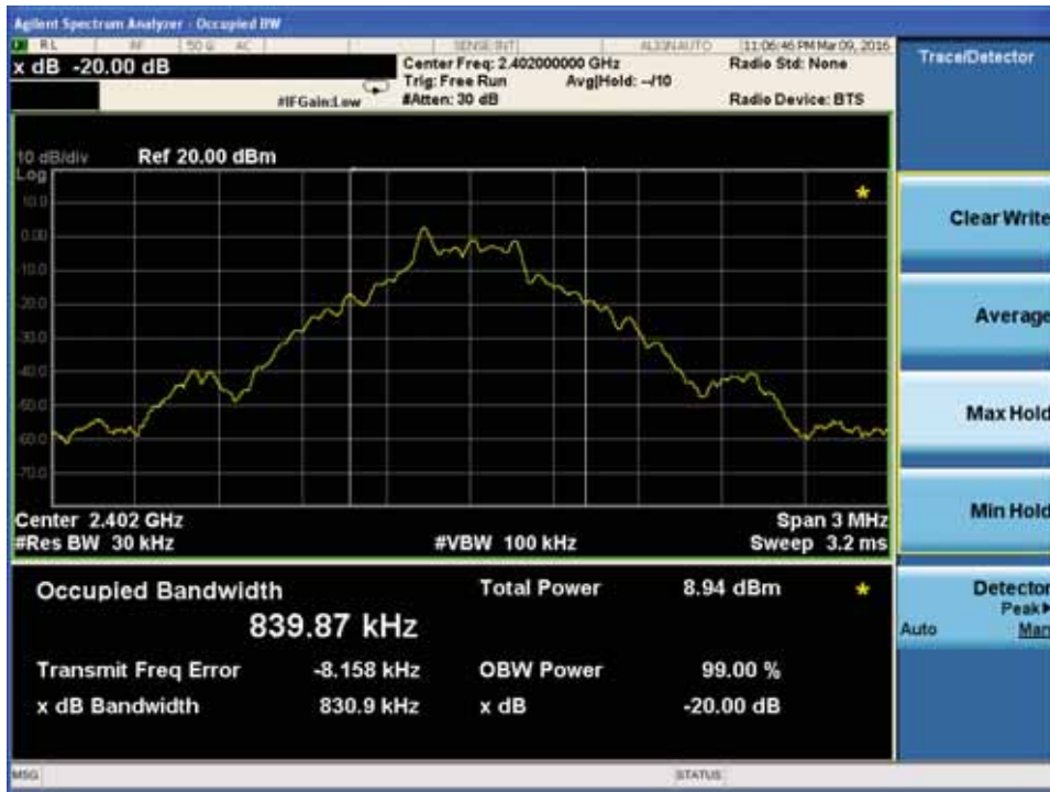
20dB Bandwidth plot on channel 39
