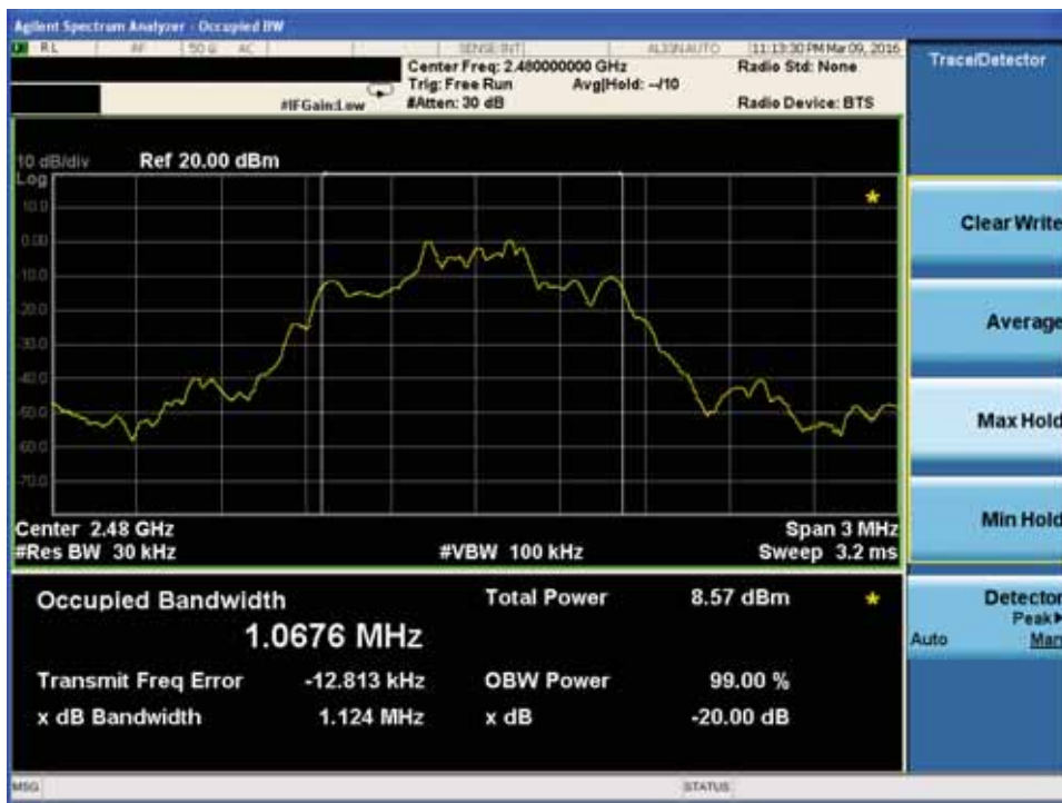
20dB Bandwidth plot on channel 78
