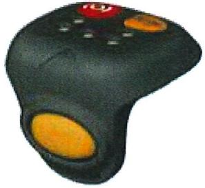
The HD4100 called a "trigger" is a wearable transceiver which also is a Bluetooth system. It has an internal capacitor that stores energy instead of a battery. It is used as a remote to operate a truck as the operator is wearing this unit.
