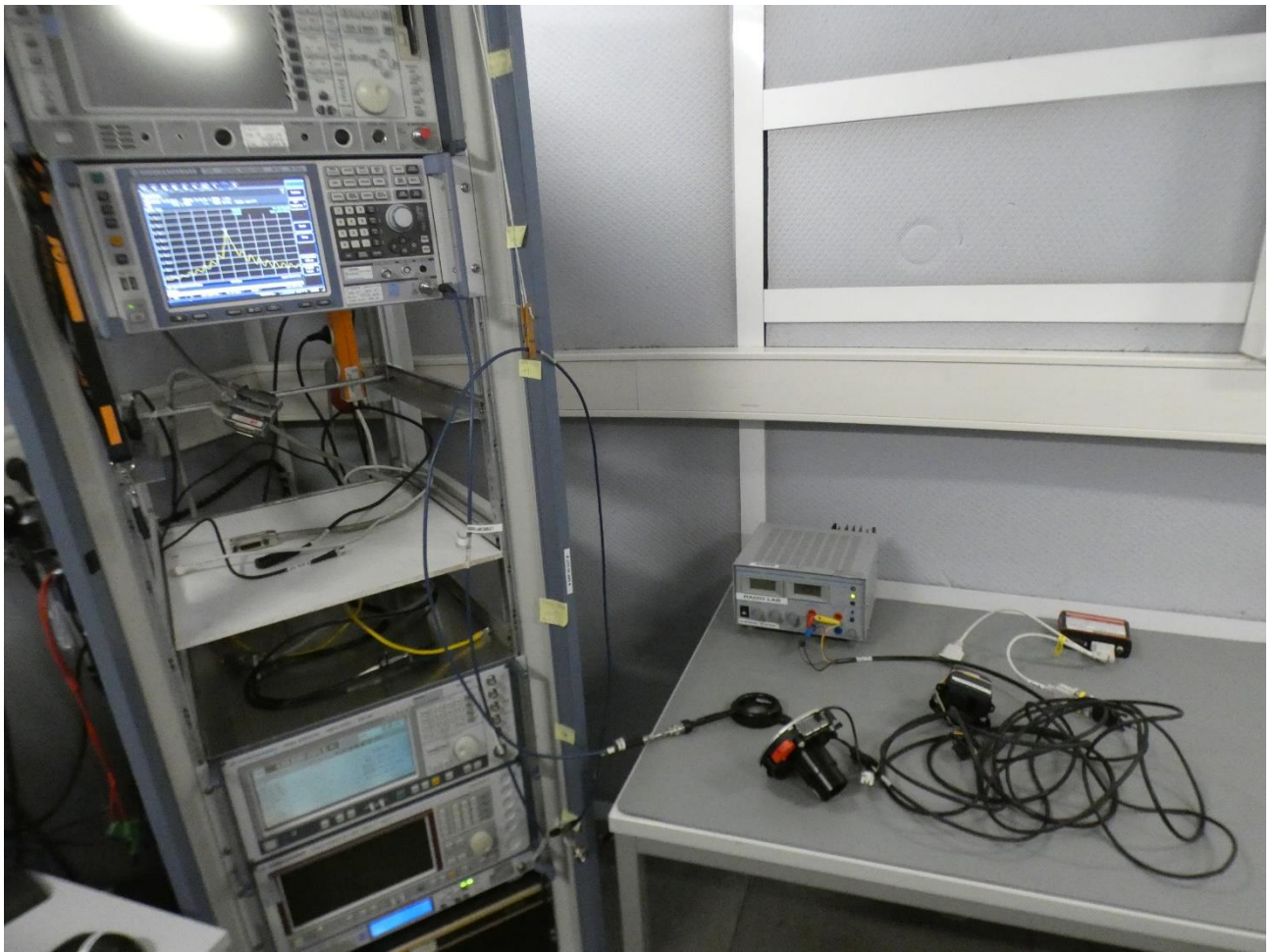
Photo 6: Test setup for conducted measurements on Radio Lab
