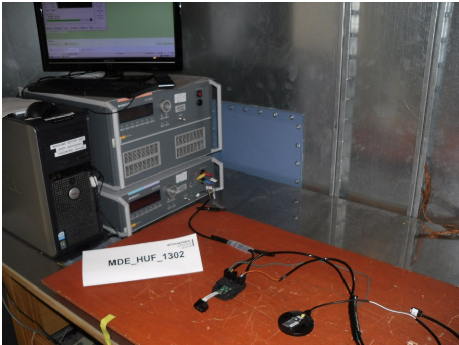
Picture 10 : setup for the test "Vehicular Pulses / Transients and Surges"
