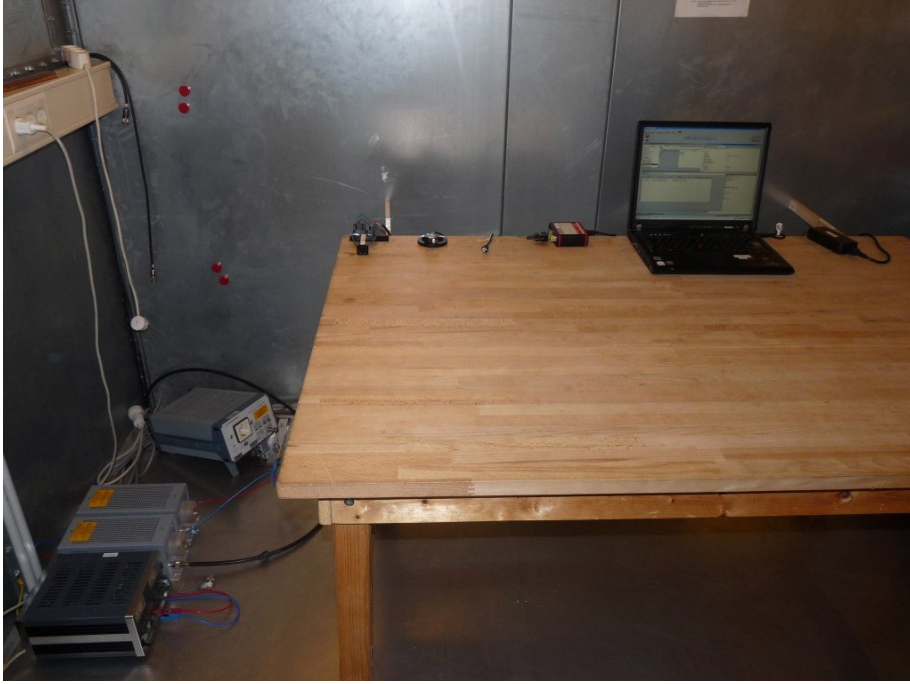
Picture 3 : setup for the test "Conducted interference voltage"
