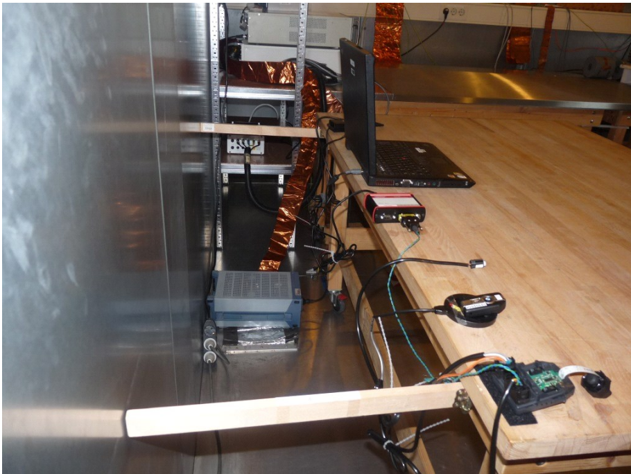
Picture 4 : setup for the test "Conducted interference voltage", detailed view
