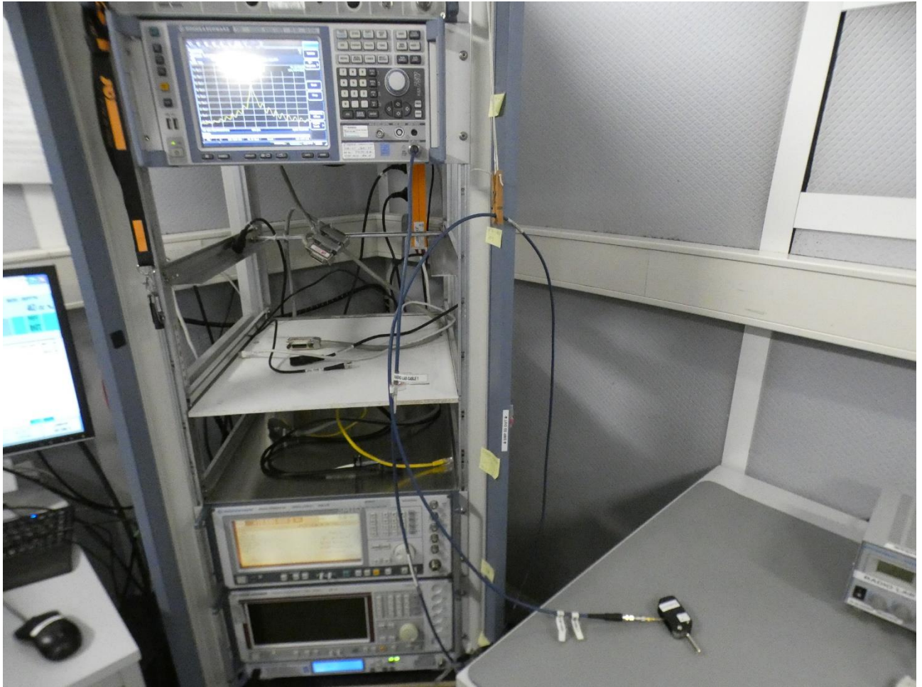
Photo 5: Test setup for conducted measurements on Radio Lab
