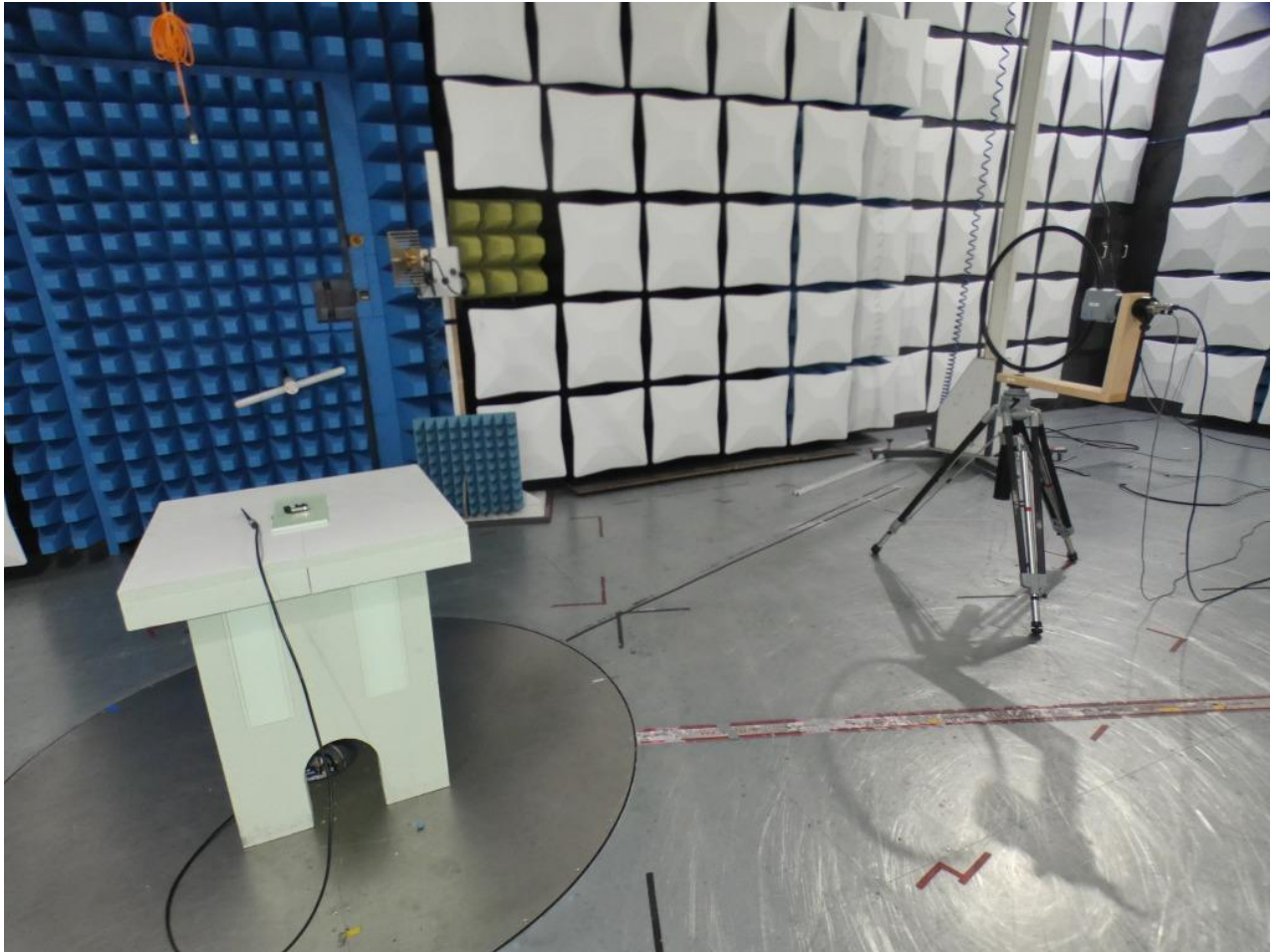
Photo 1: Test setup for radiated measurements (9 kHz - 30 MHz)
