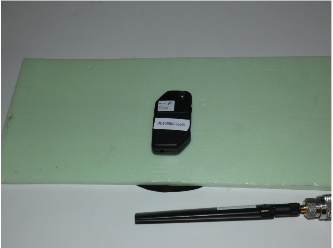
Photo 4: Test setup for radiated measurements, EUT
