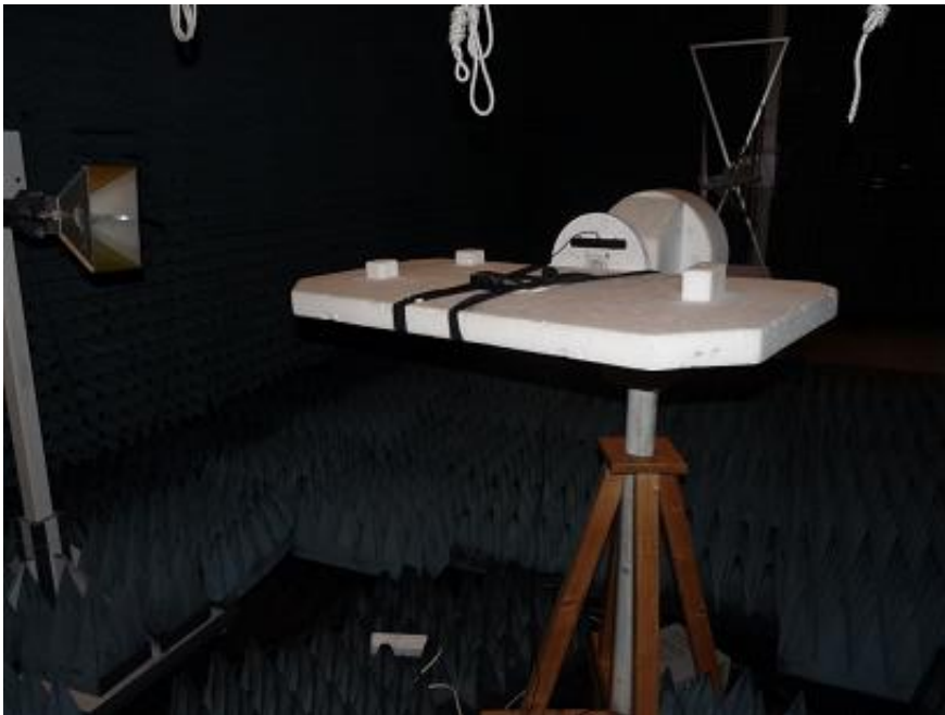
Photo 2: Setup for radiated emissions test
