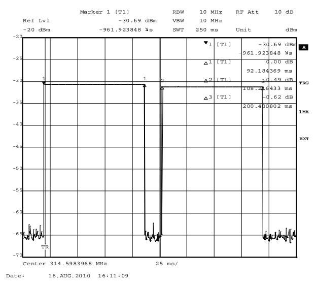
Step 2: 250 ms sweep, cycle to determine the on/off ratio within 100 ms
