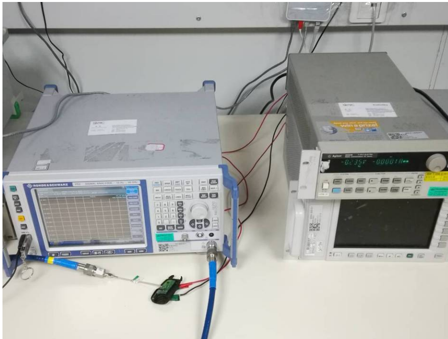
Conduction Emissions Test Setup
