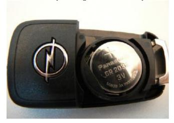
Do not touch the printed circuit board or the PCB battery holder. To reassemble the transmitter case, snap the battery box cover to the housing lower shell. Make sure that the battery box cover reliably engage.
