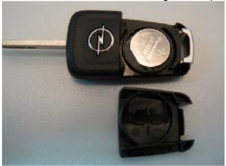
Remove the old battery from the PCB battery holder.
