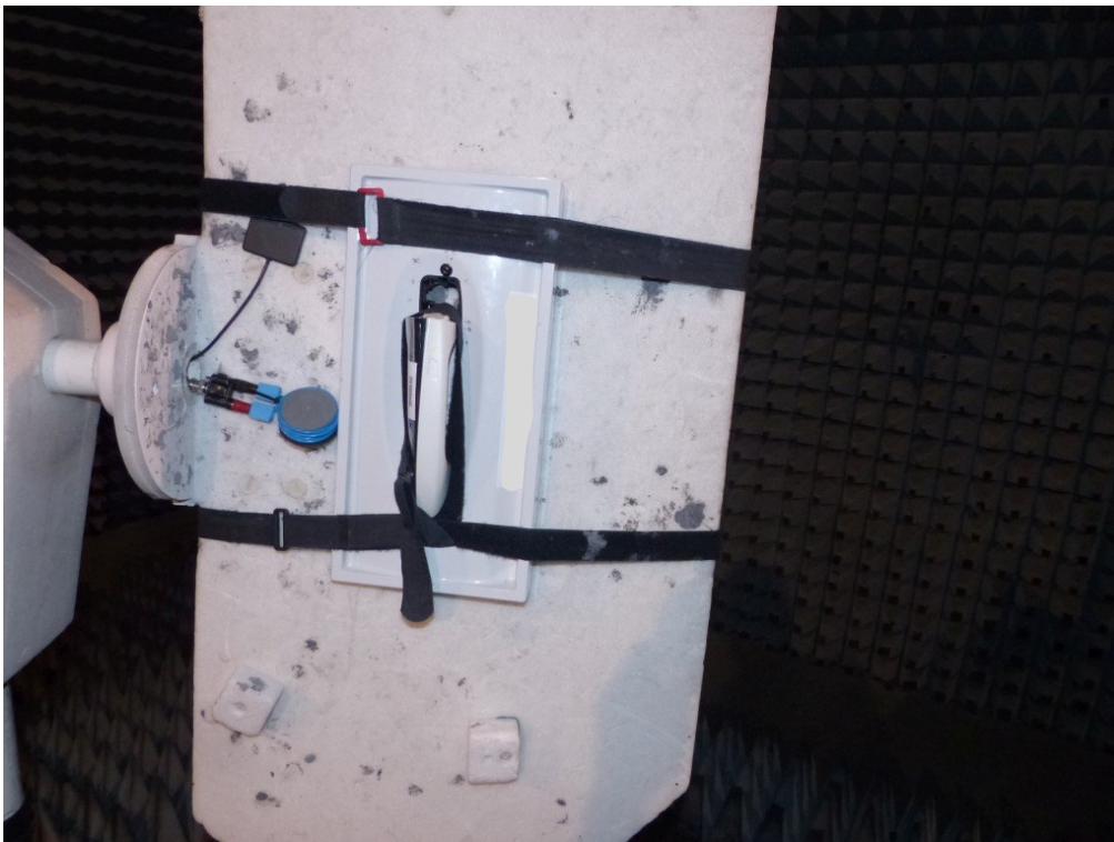
Photo No. 4: Setup for radiated tests ( f \geq 30 MHz), detailed view
