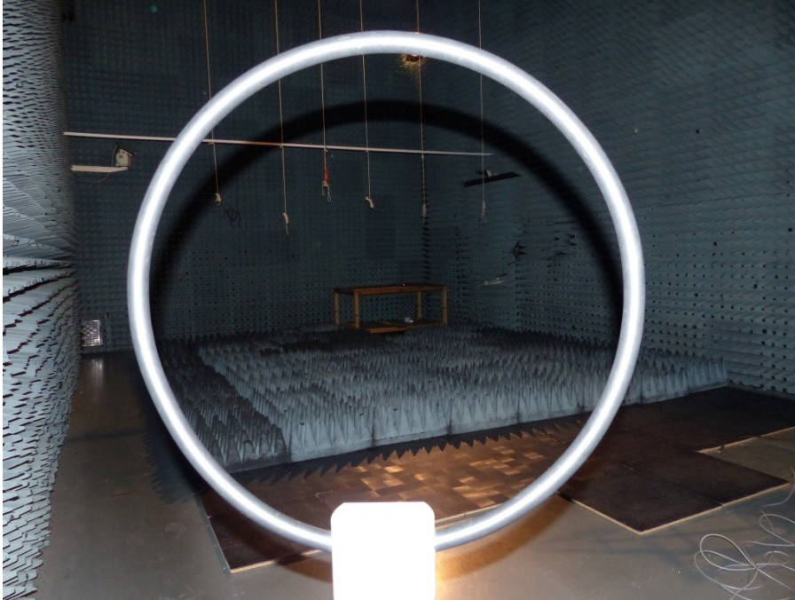
Photo No. 1: Setup for radiated tests ( f < 30 MHz), general view
