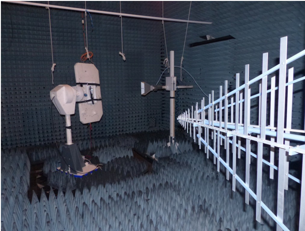
Photo No. 3: Setup for radiated tests ( f \geq 30 MHz), general view
