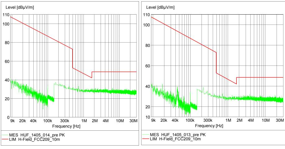
TX on 314.0 MHz, CH:1, Antenna position 0° left side, horizontal EUT position
