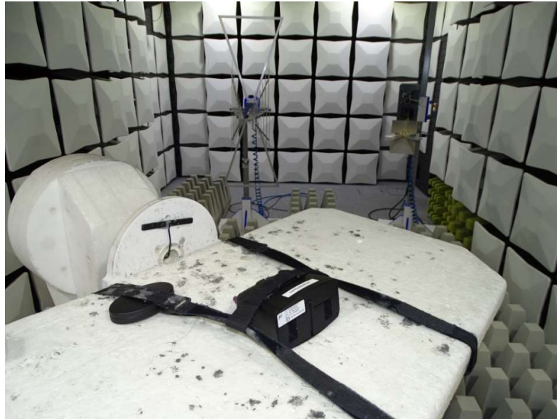
Photo 3: Test setup for radiated emissions measurements in fully-anechoic chamber (1 GHz to 26 GHz), front side view
