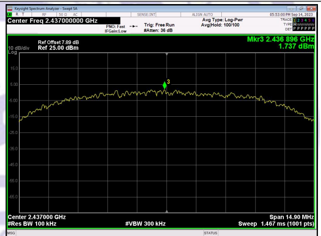
In-Band Reference Level IEEE 802.11b_Channel 6_20MHz_Antenna 0
