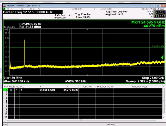
In-Band Reference Level IEEE 802.11g_Channel 11_20MHz_Antenna 0
