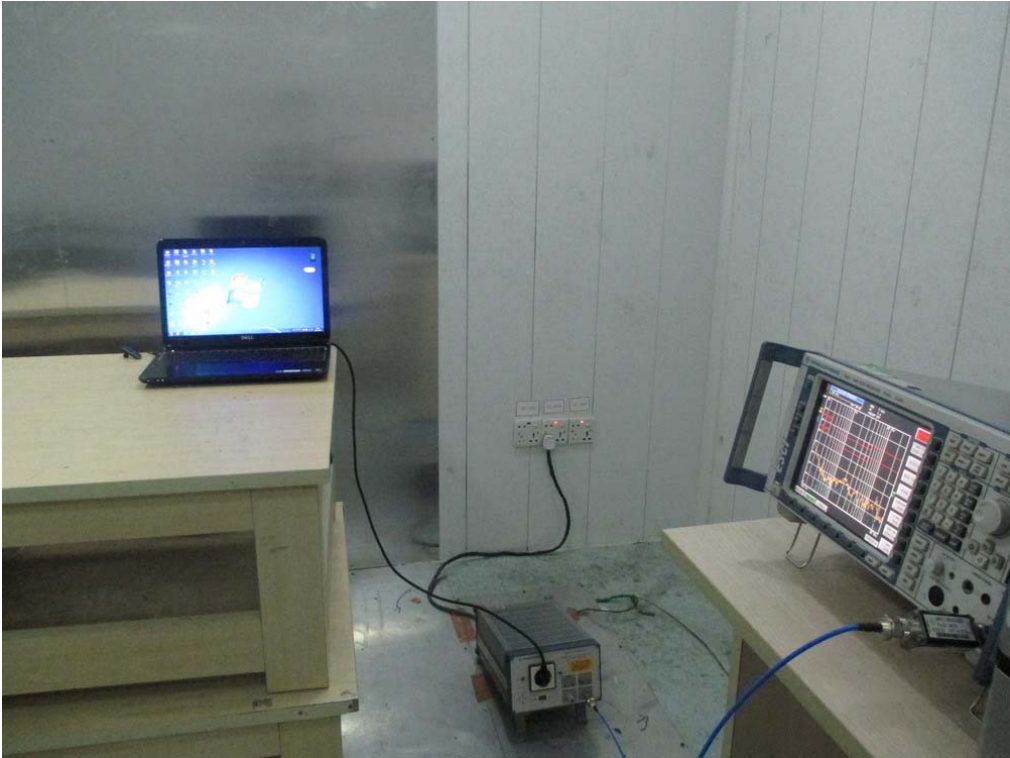
FCC RADIATED EMISSION TEST SETUP
