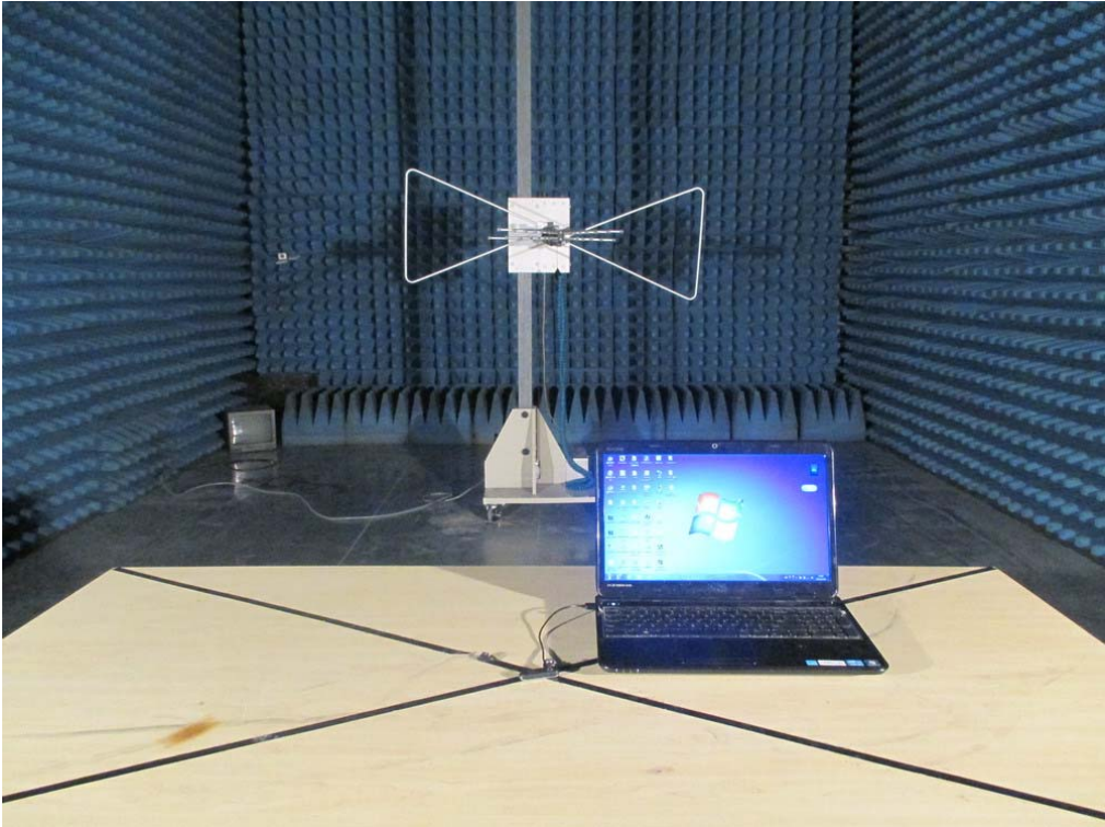
FCC RADIATED EMISSION TEST SETUP
