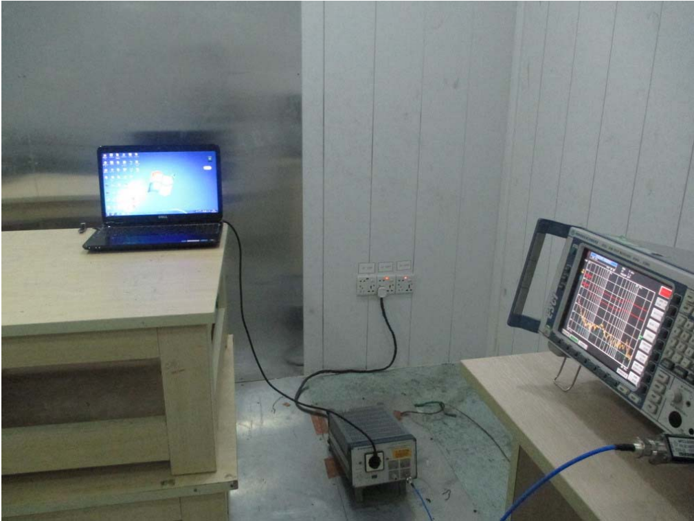
FCC RADIATED EMISSION TEST SETUP
