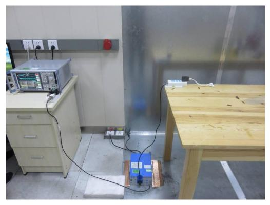
FCC RADIATED EMISSION TEST SETUP
