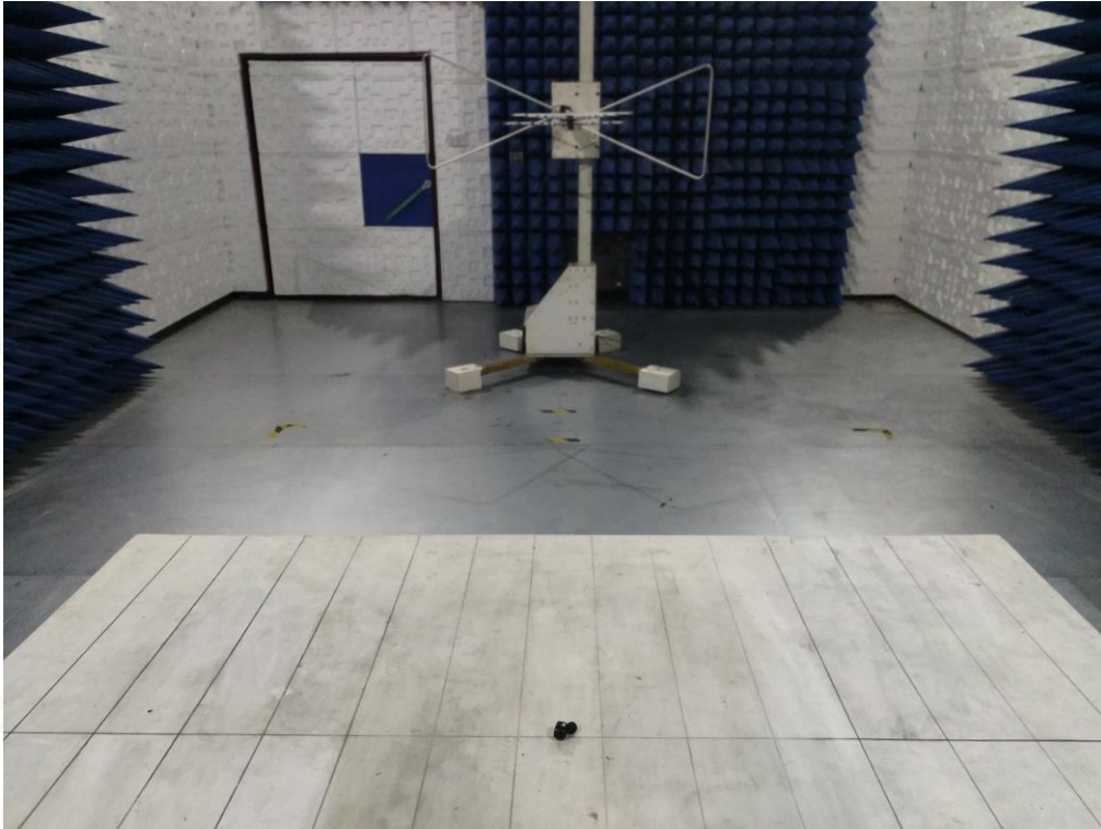
RADIATED EMISSION TEST SETUP ABOVE 1GHZ
