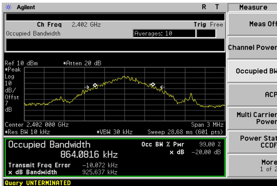
**20dB Bandwidth & 99% Bandwidth Test Data CH-Mid**
