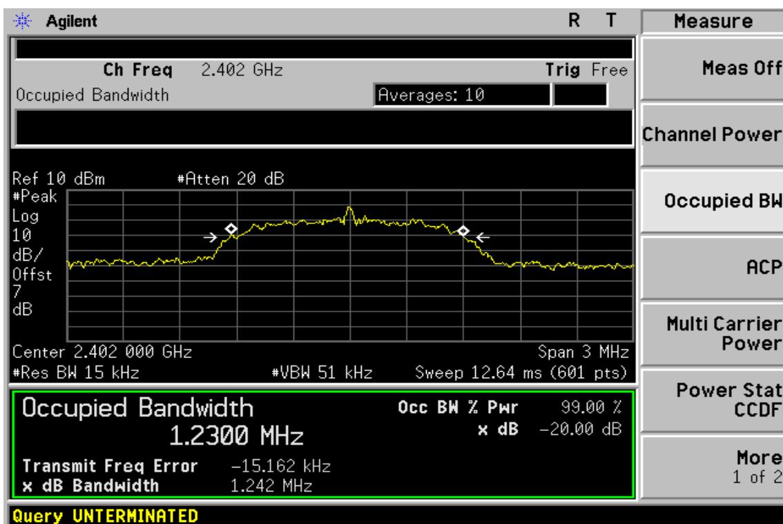
**20dB Bandwidth & 99% Bandwidth Test Data CH-Mid**
