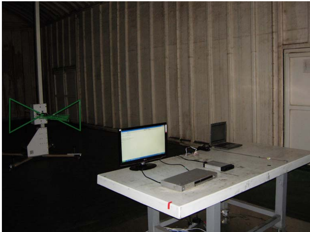
Back View of Radiated Test (Bilog)
