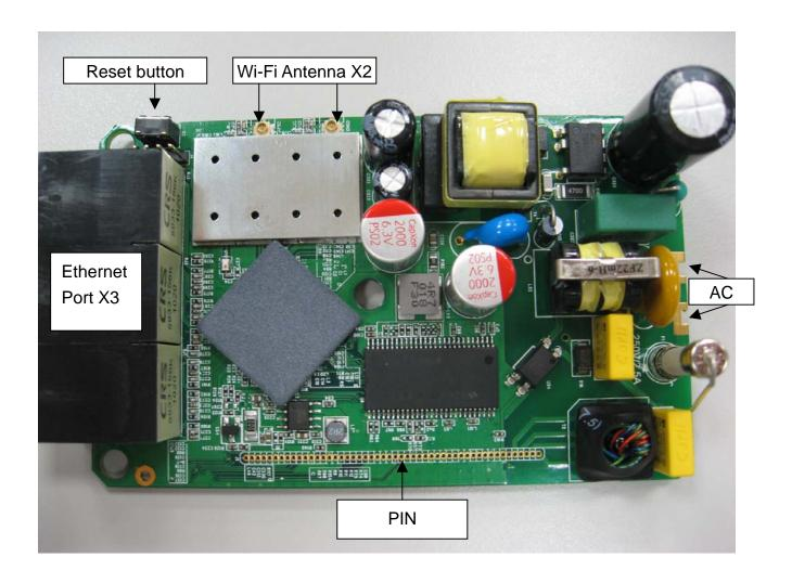
Reset Button: Press Reset button to revert it to factory default.
