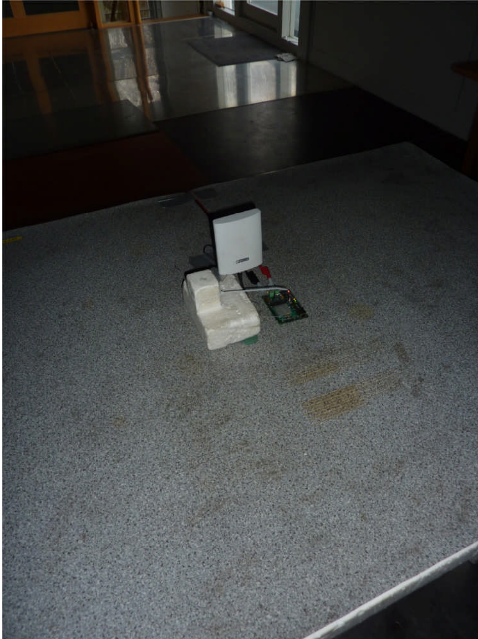
114368_13: Test setup open area test site (patch antenna)
