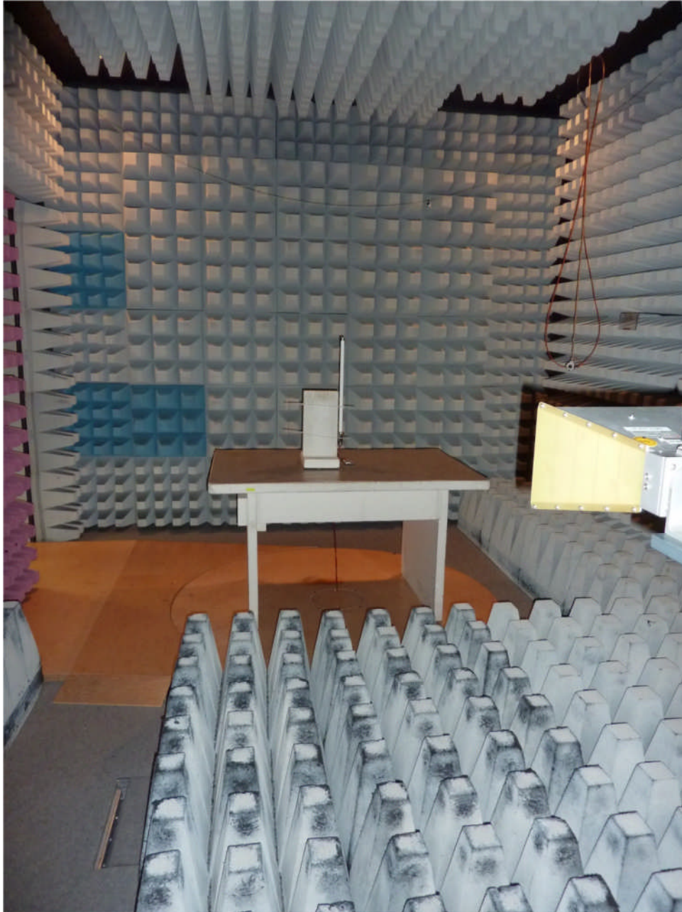
114368_07: Test setup fully anechoic chamber (monopole antenna)
