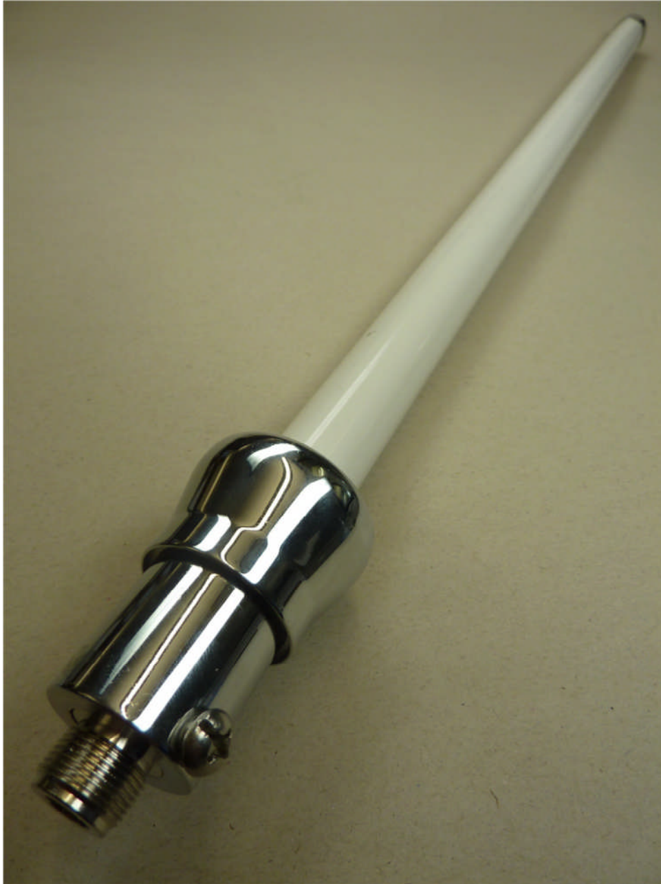
114368_EUT14: Monopole antenna, 3D view
