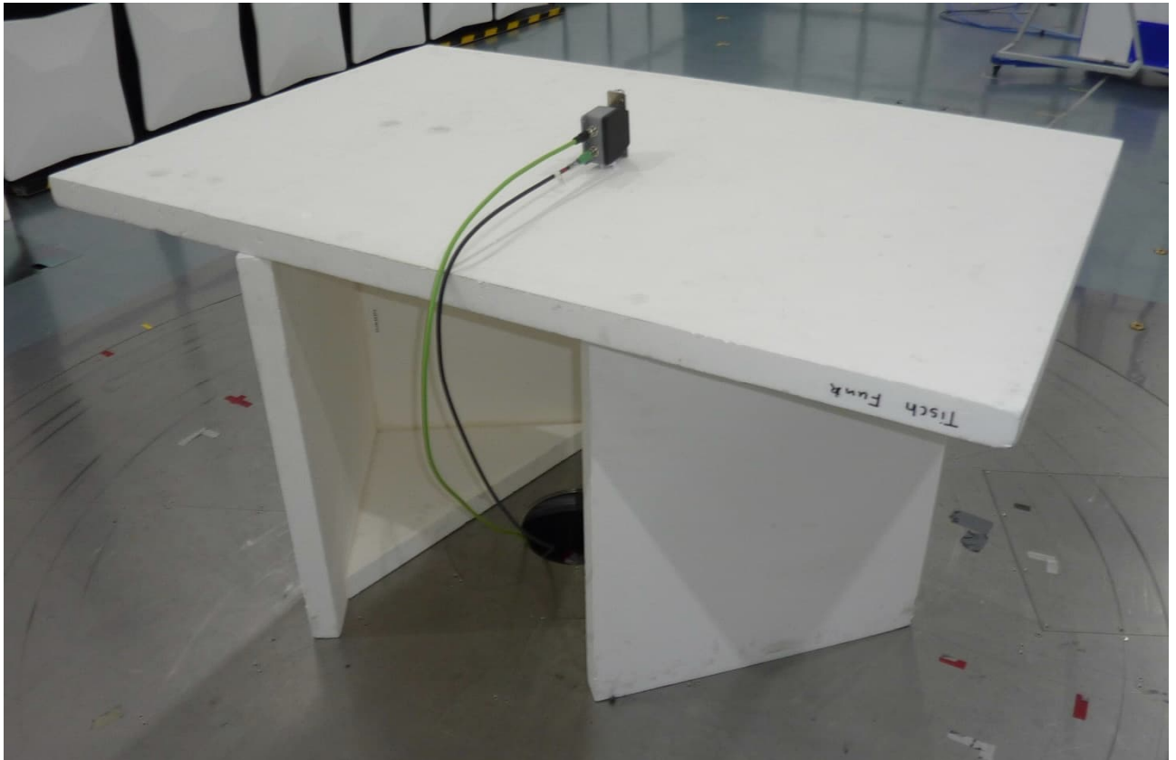
Test setup - Radiated emission (semi anechoic chamber)
