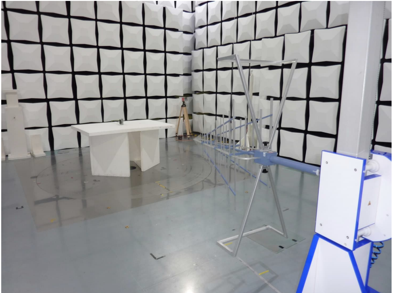
Test setup - Radiated emission (semi anechoic chamber) 30 MHz – 1000 MHz
