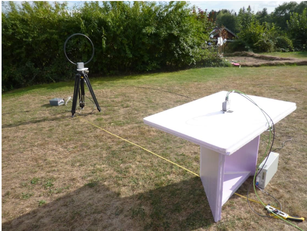
Test setup - Radiated emission (Outdoor test side)
