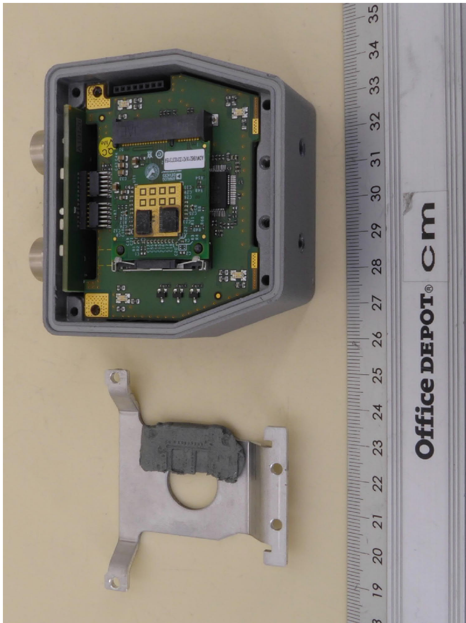
NEARFI PD 2A ETH R, internal view 2, shielding removed
