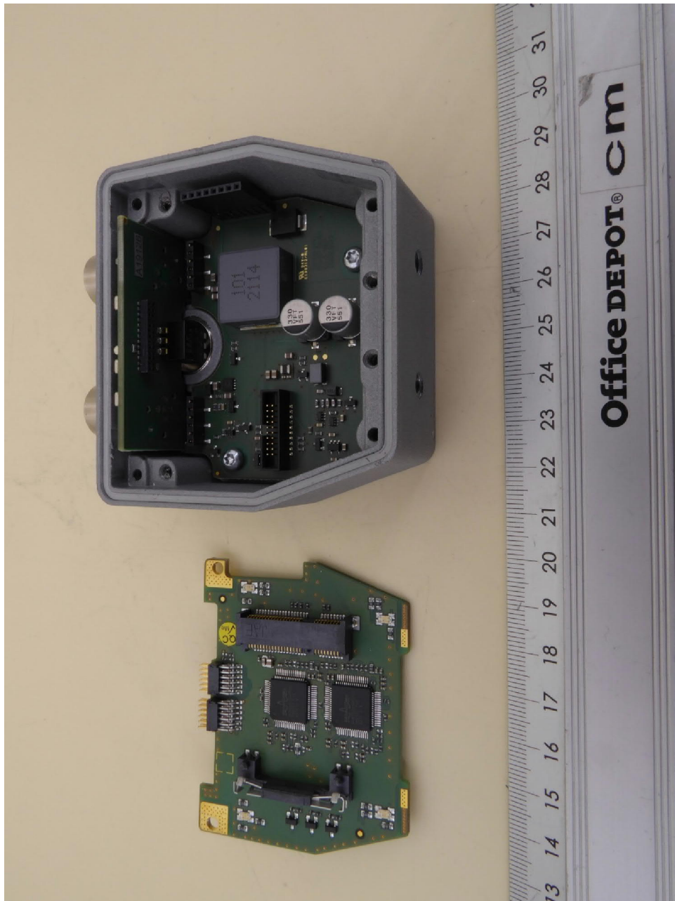
NEARFI PD 2A ETH R, internal view 4, data PCB removed
