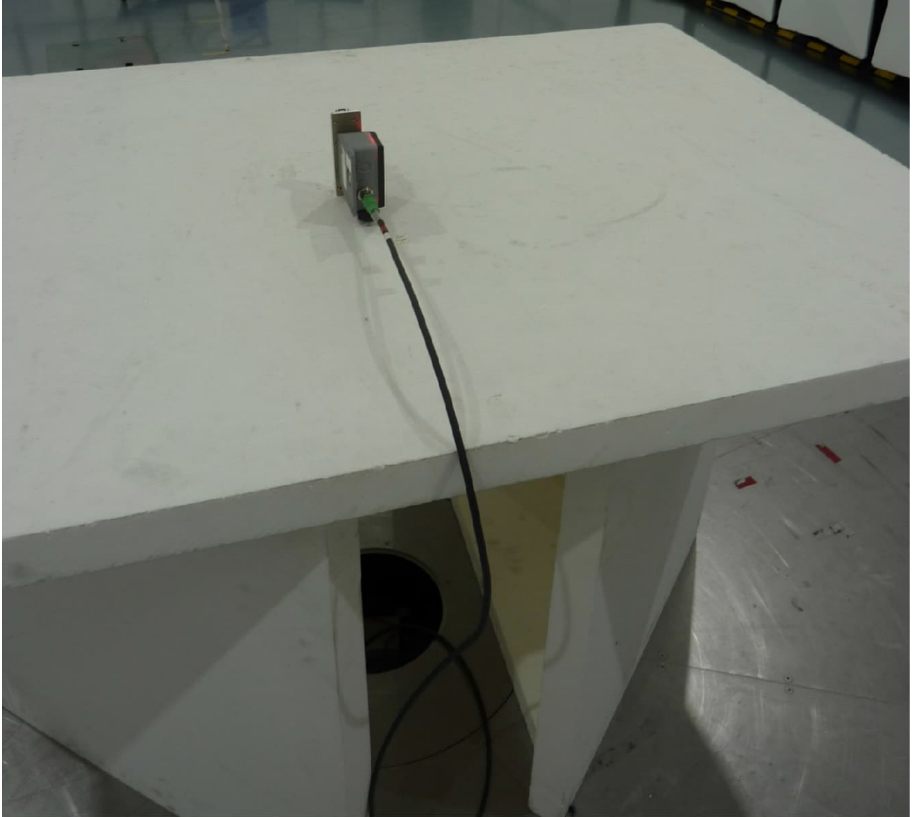
Test setup - Radiated emission (semi anechoic chamber)
