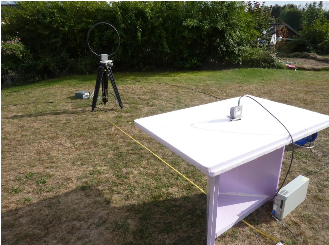
Test setup - Radiated emission (Outdoor test side)
