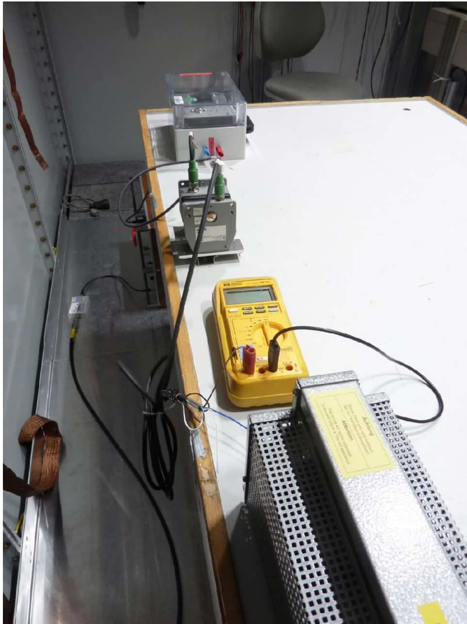
Test setup – Conducted emissions on power supply lines - base (EUT) and remote (client) unit
