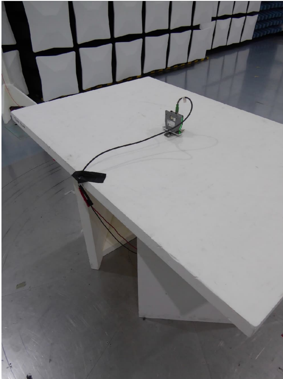
Test setup semi anechoic chamber (position 1)
