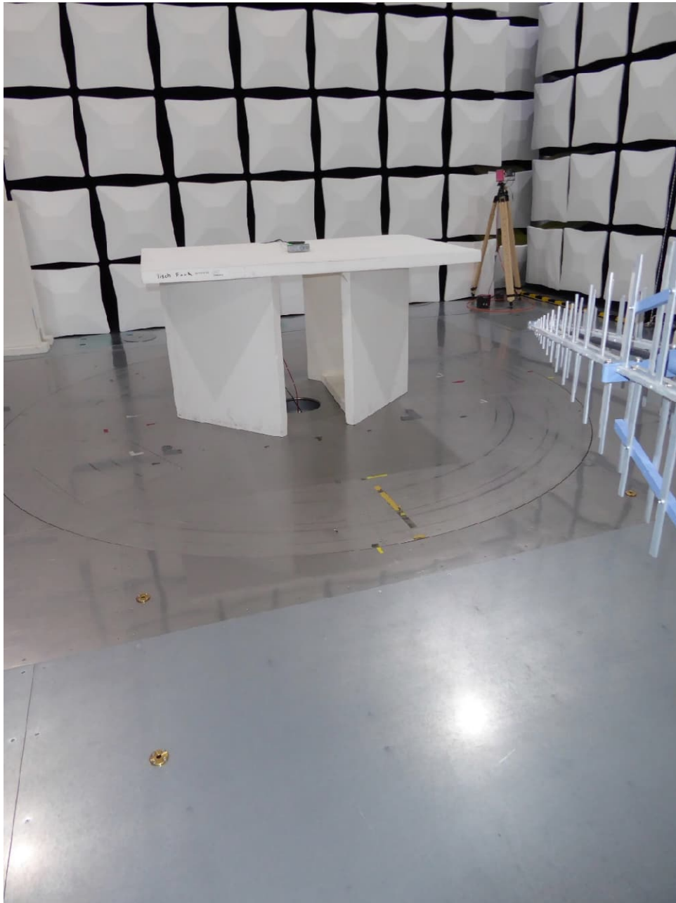
Test setup semi anechoic chamber <1 GHz
